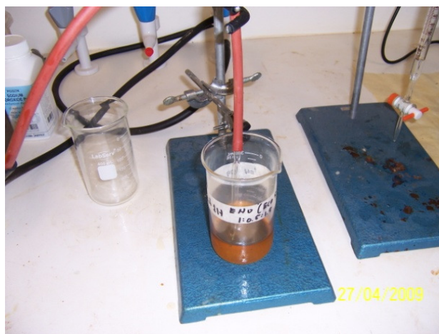
Figure 17 The sample is dried by bubbling air up through the resin.
