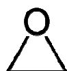
Figure 6 Oxirane ring, otherwise known as an epoxy group. The oxirane oxygen content refers to the content of the oxygen atom present in the group.
