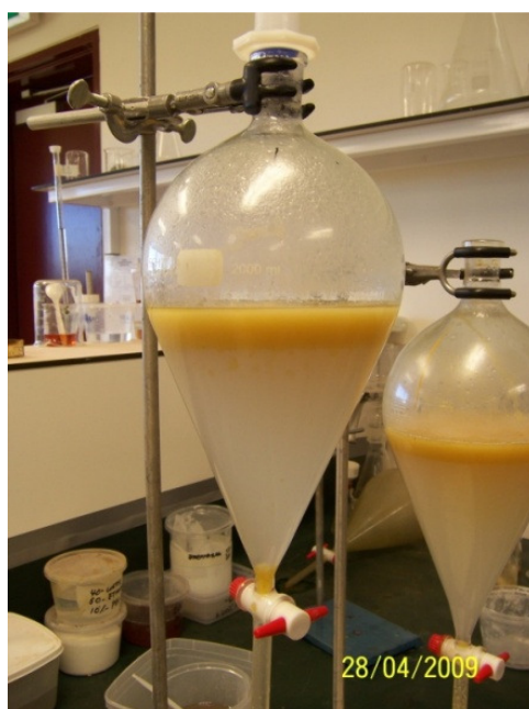
Figure 14 A washed batch of resin usually looks like that in the picture, with a resin phase on the top, a relatively clear aqueous phase in the middle and the AIER on the bottom.
