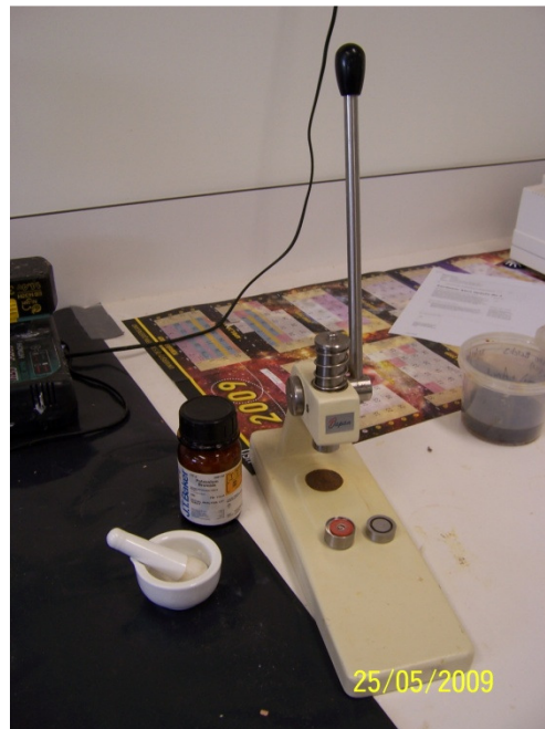
Figure 18 Equipment for making a FTIR sample plate
