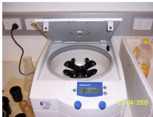
Figure 16 The centrifuge, used to separate the aqueous phase from the oil phase after washing
