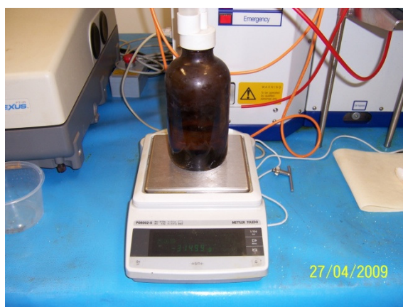
Figure 11 As the hydrogen peroxide is dosed the scales register a negative value. It is worth checking this value after the dosing stage is complete to ensure the correct amount has been administered.
