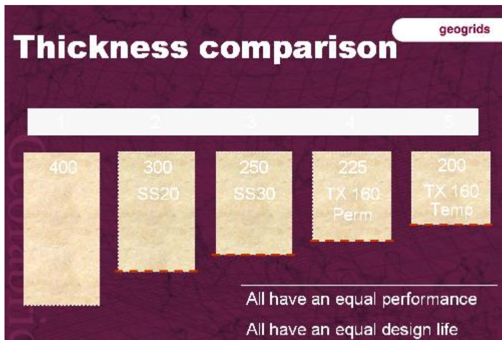
Figure 7.8: Thickness comparison of Geogrids to gravel (Geofabrics Australia 2009)
