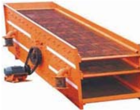
Figure 16: Vibrating Screen General Assembly (Malco 1986)
