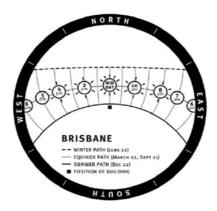
Figure 12: Brisbane Sunpath Diagram
