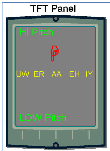
Figure 10 Mapping a TFT Panel to Vowels and Pitch (Altium Ltd. 2009, NB2 TFT Panel Port Plug-In Library Component).
