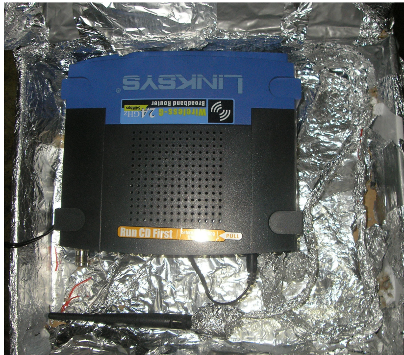
Figure 5.2: Photo showing the inside of the box housing the router
