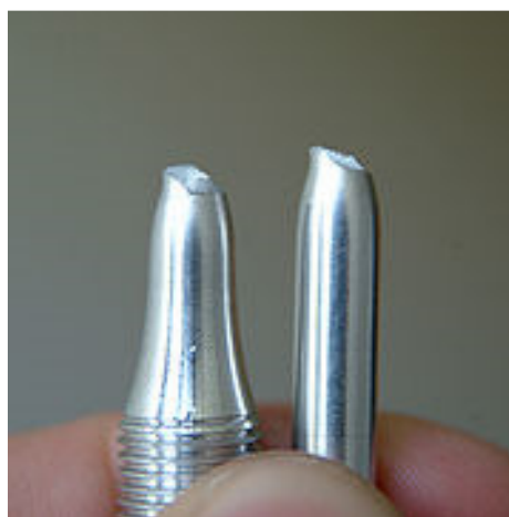
Figure 24 - Metal Alloy Necking
