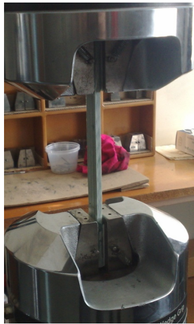
Figure 21 - Coupon Undergoing Tensile Test
