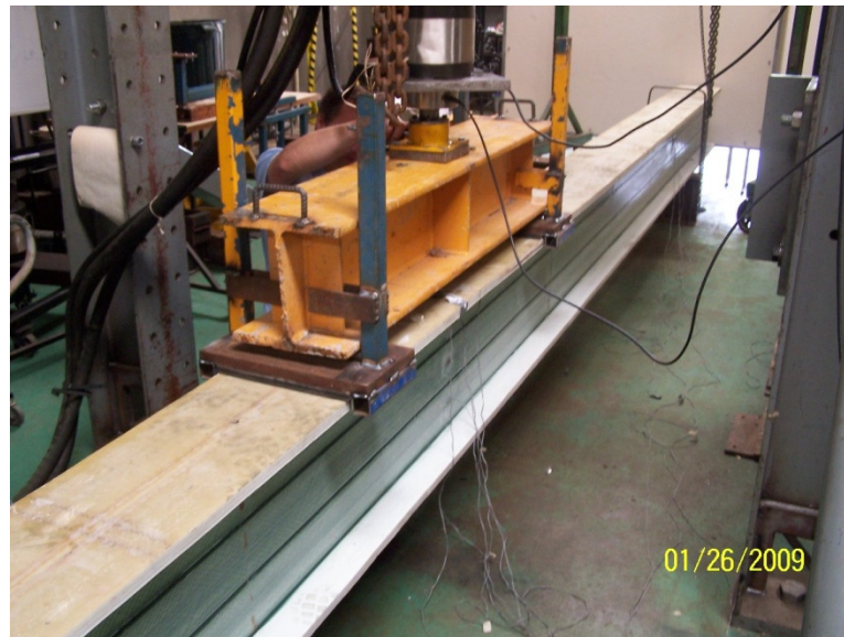
Figure 29 - Composite Girder Undergoing Fatigue Testing
