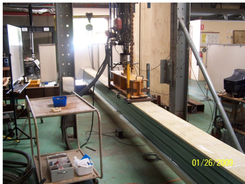
Figure 19 - Bending Fatigue Test Setup
