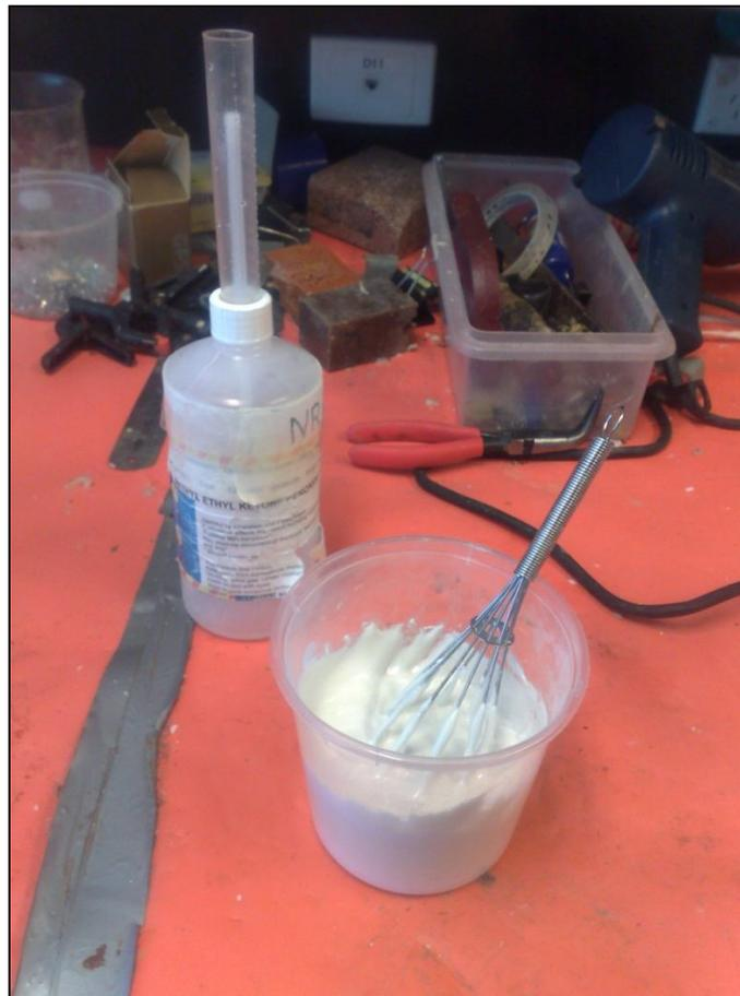
Figure 11: Mixing the resin, glass powder & MEKP.
