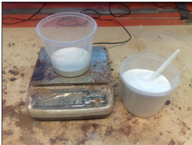
Figure 9: Weighing the glass powder.
