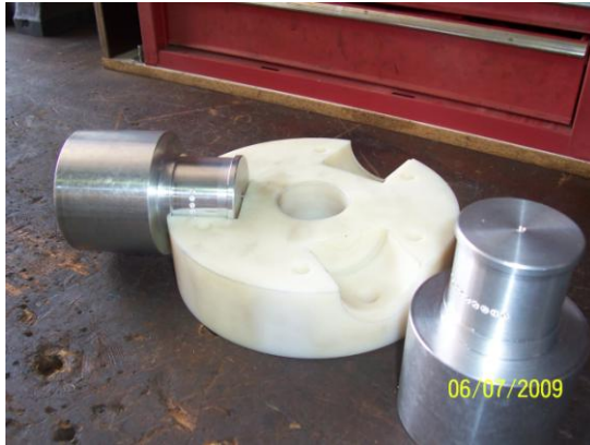
Machined nylon hub and unfinished blade root holders
