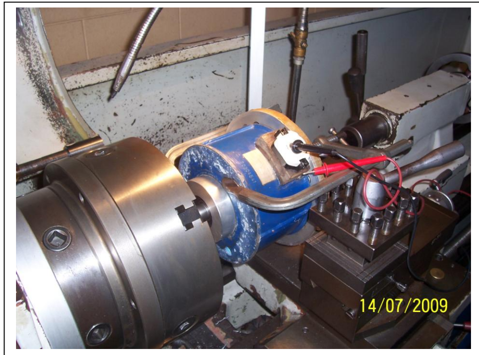
Fig 4.14- Generator mounted in jaws of lathe chuck
