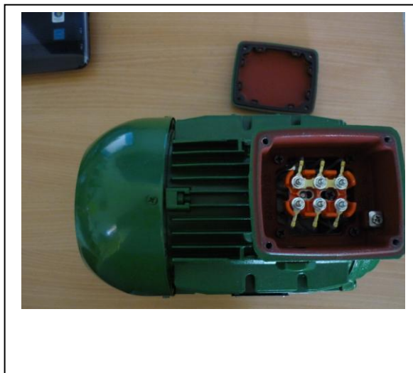
Fig 4.4- generator circuit box
