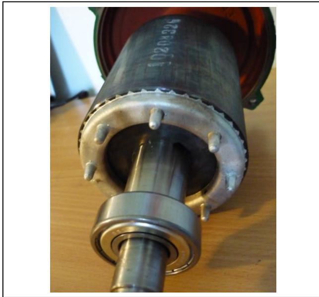
Fig 4.3 -Generator rotor, shaft , and bearing
