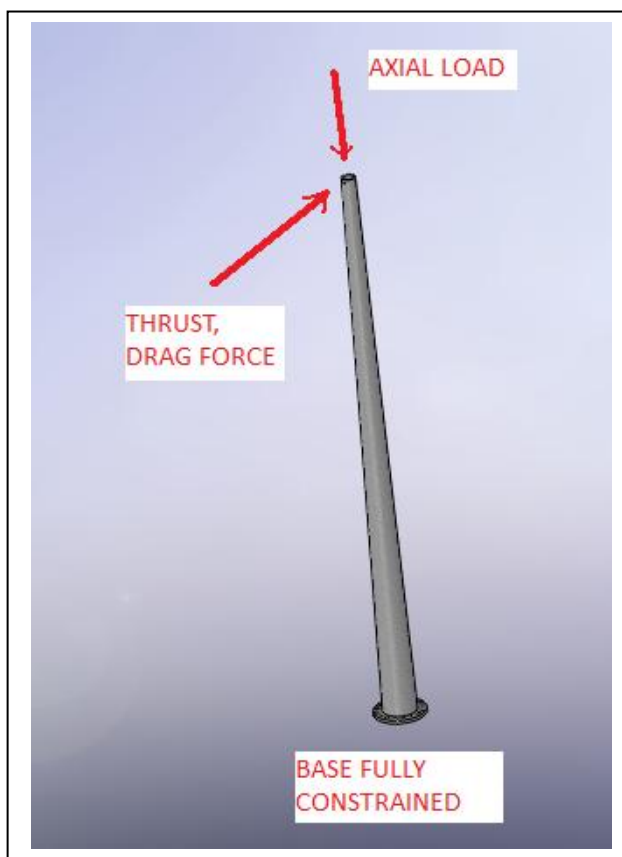
Figure A4 - Loading of tower
