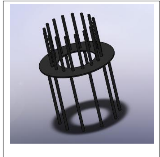
Fig 5.14- Steel reinforcing and anchor studs
