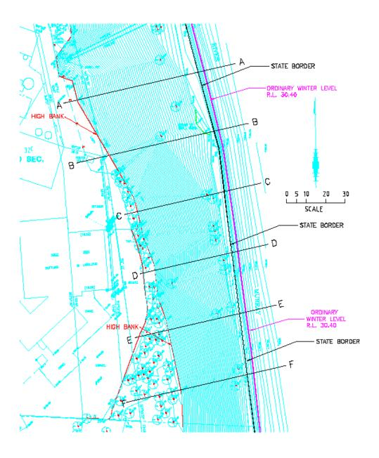
The cross section levels located at Site 1 produced results very similar to what I had expected. The high bank located just above the fixing of the ordinary winter level is of a similar offset distance along the entire 300 metre survey area.
