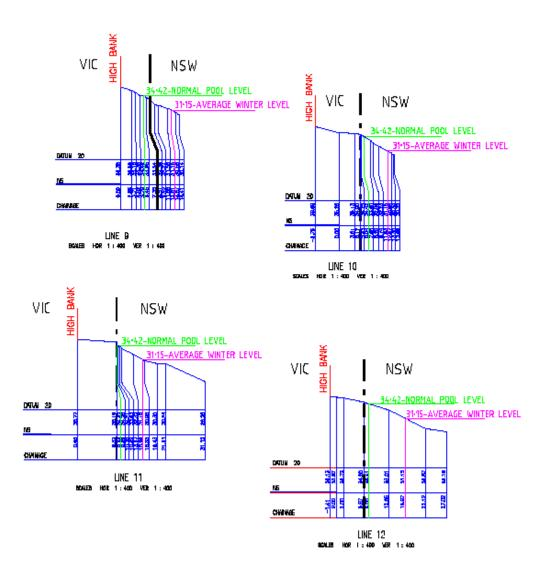
**Appendix E** (Examples of two sheets of the complete 49 sheet set of plans now supplied to assist surveyors in the re-establishment of the state border.)
