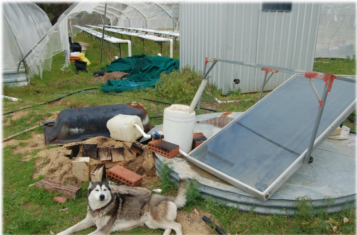
Figure 4-7: Attempt to maintain even temperature by submergence in aquaponics tank. Author's dog supervising work. Note previous attempt at water heating with a steel bathtub and fire.
