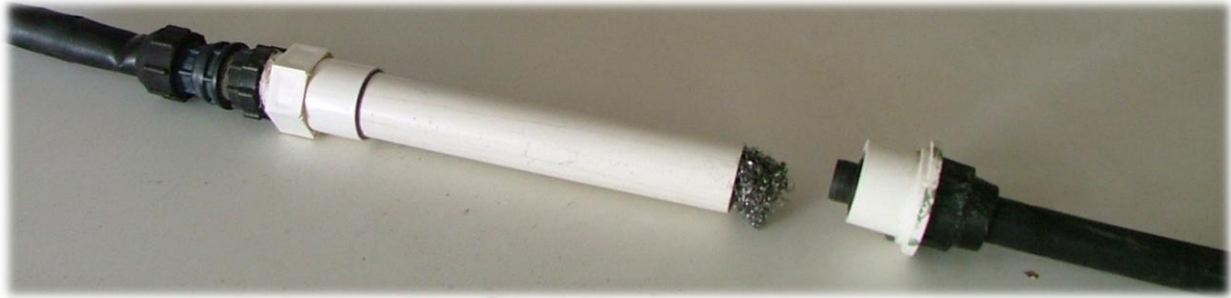
Figure 4-7: H 2 S oxidation scrubber
