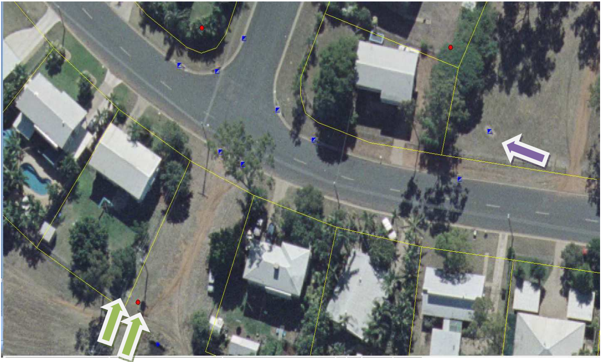
Figure 9.4: Aerial photo with the locations of stormwater pits and sewer manholes to perform spot checks. The arrows indicate the actual and data base locations of the assets.
