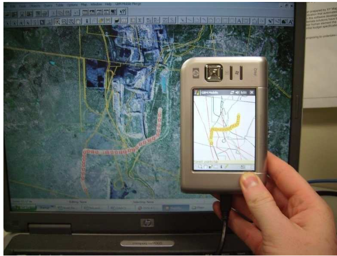
Figure 8.3: PDA with GMB Mobile software compared to the image of MapInfo on the screen behind.
