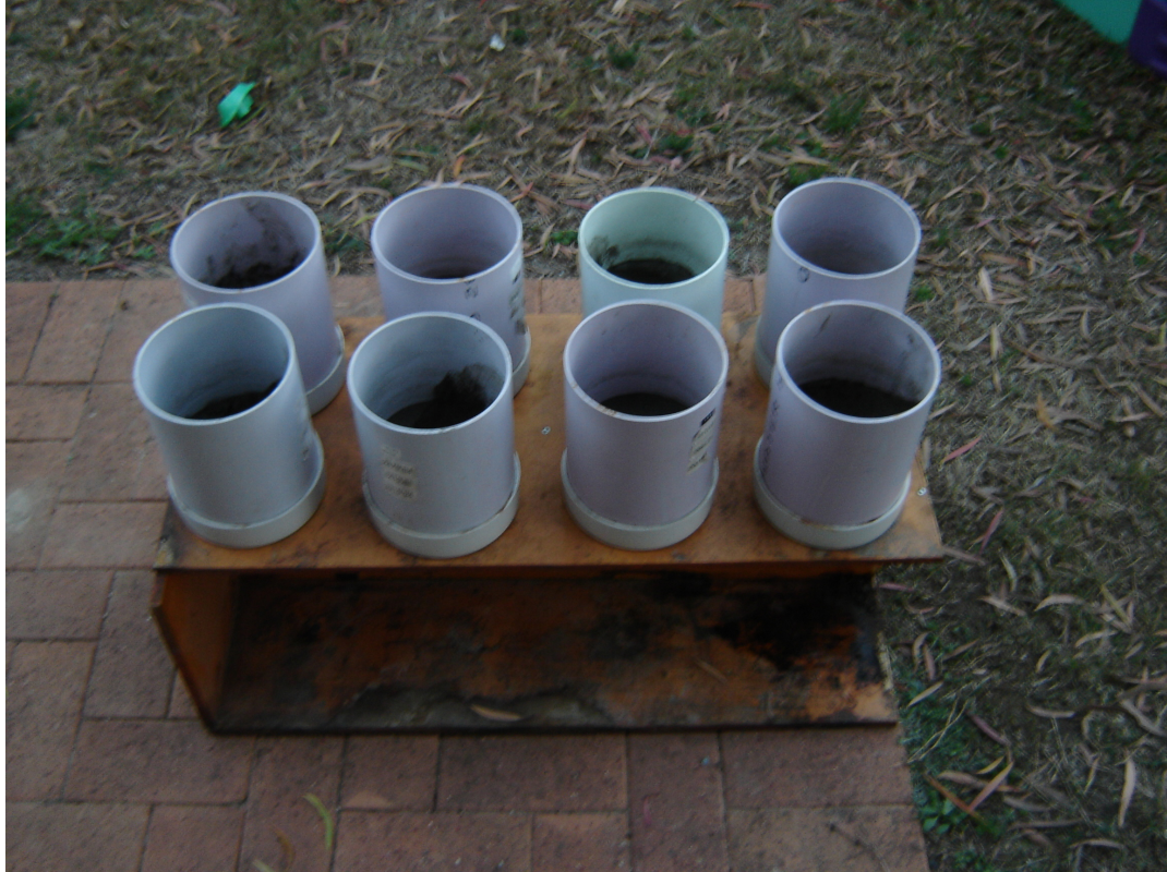
Figure 5.3: Photograph of leaching columns in holding rack
