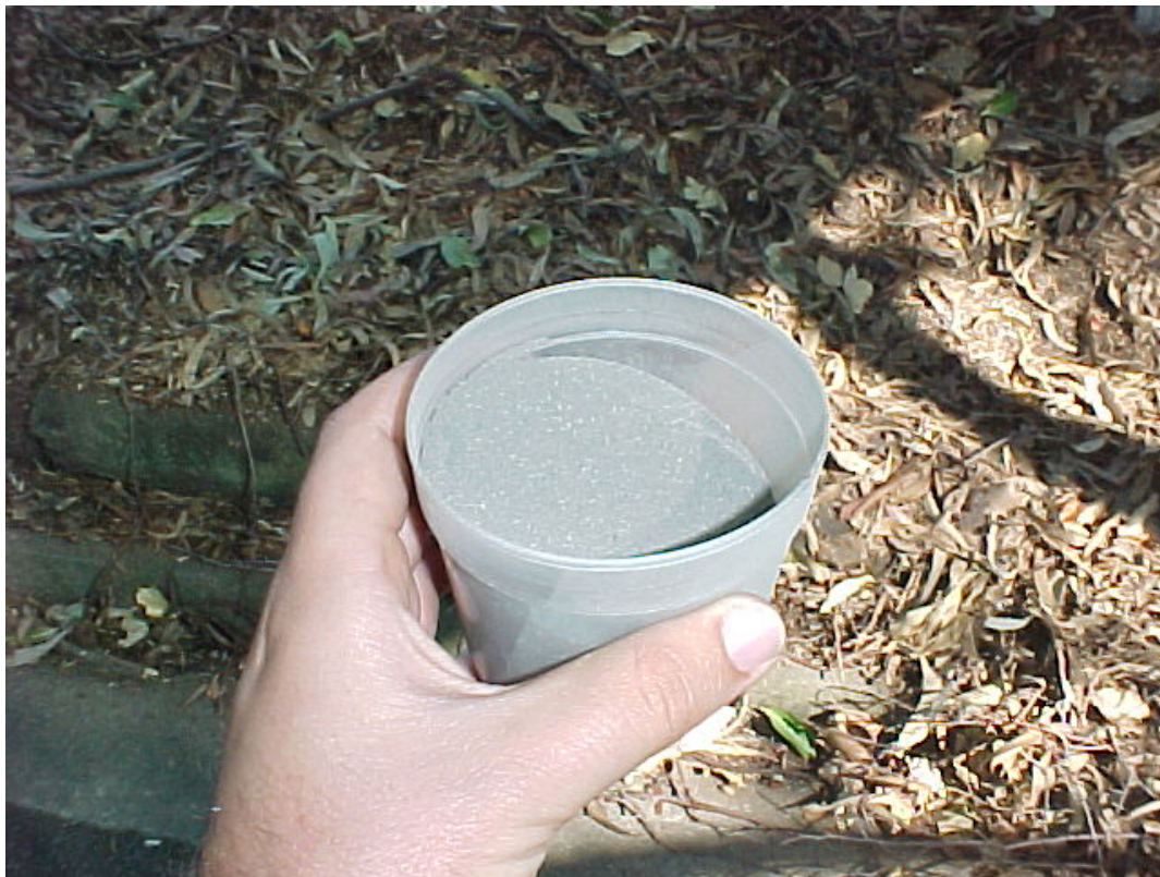
Figure 5.5: Acid Sulfate Soil sample used in the leaching column experiment
