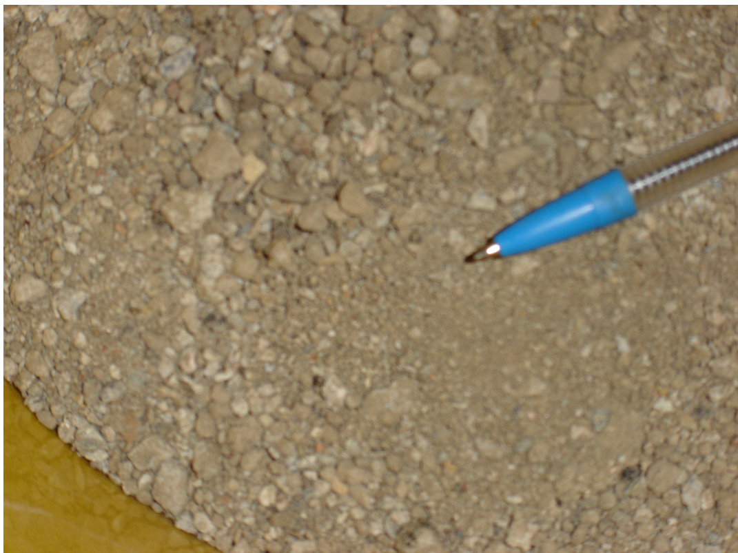
Figure 4.7: Queensland Recycling Crusher Dust close-up using pen as scale
