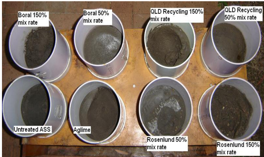
Figure 5.4: Leaching column layout, including content descriptions
