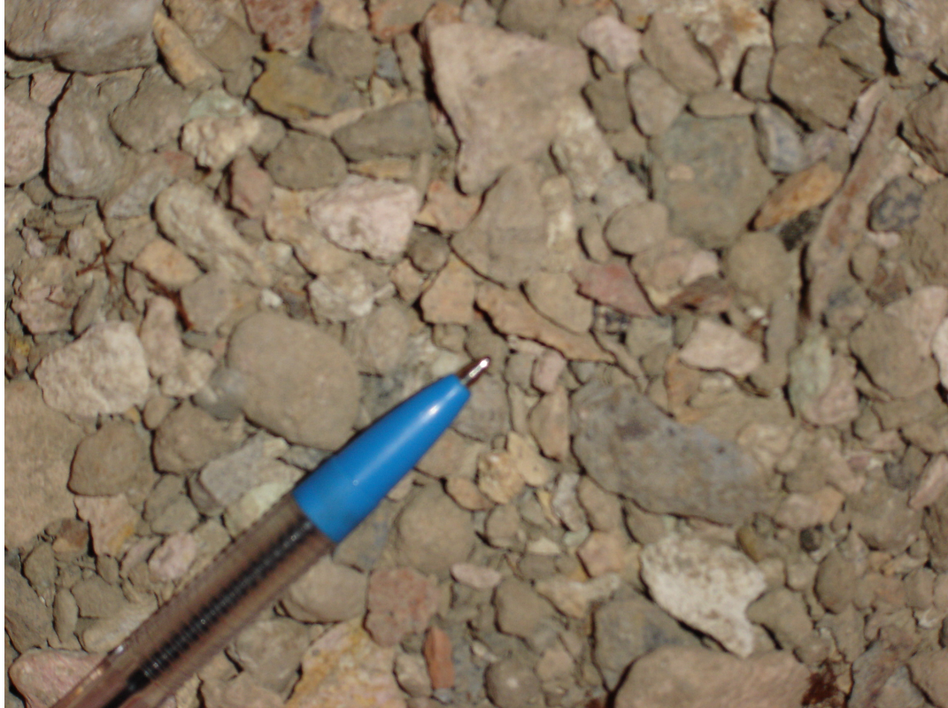
Figure 4.3: Close-up of Rosenlund crushed concrete product using pen as scale.
