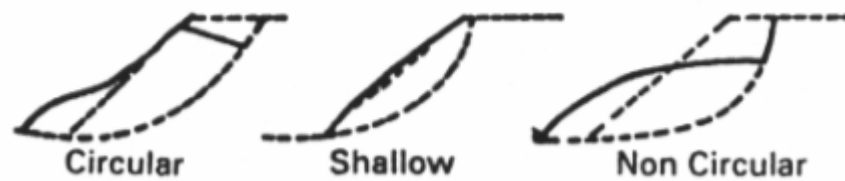
Figure 2.2 Rotational slides ( Slips & Slumps) (Raj, 1995)
