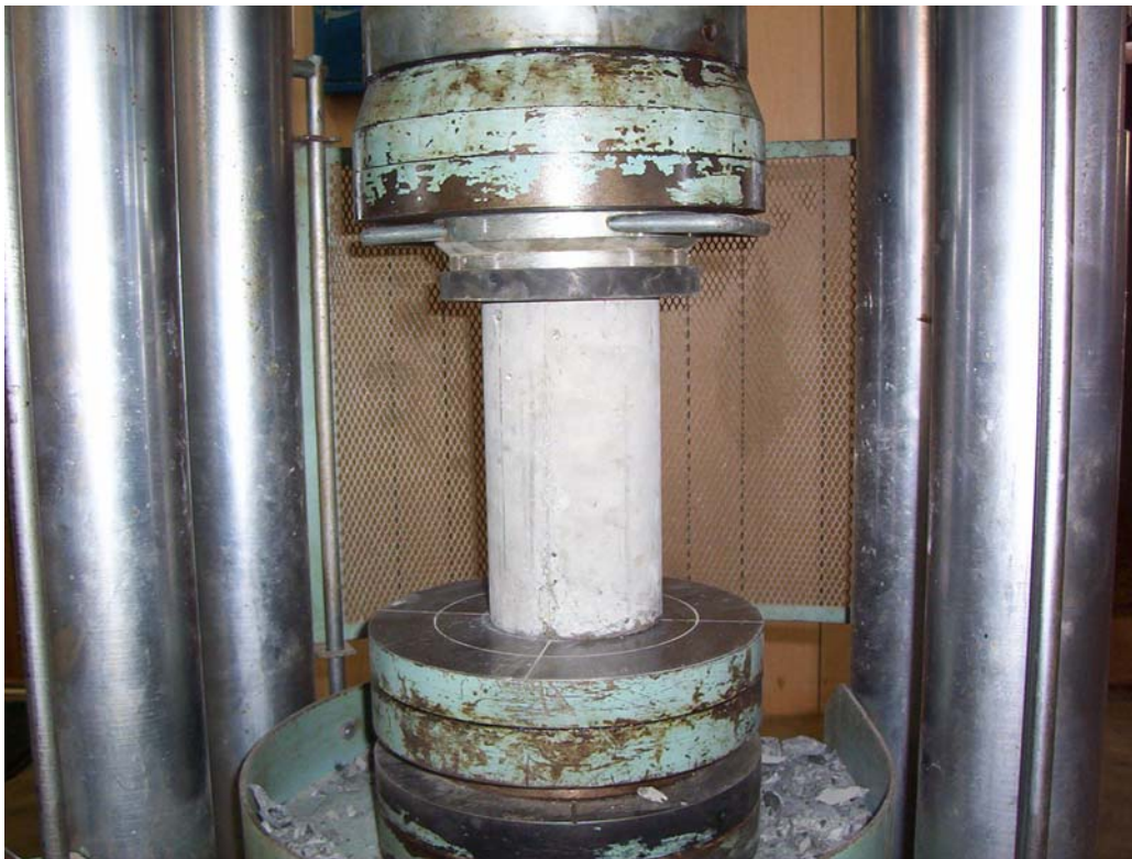
Figure 3.3: Compression cylinder capped and ready to be tested
