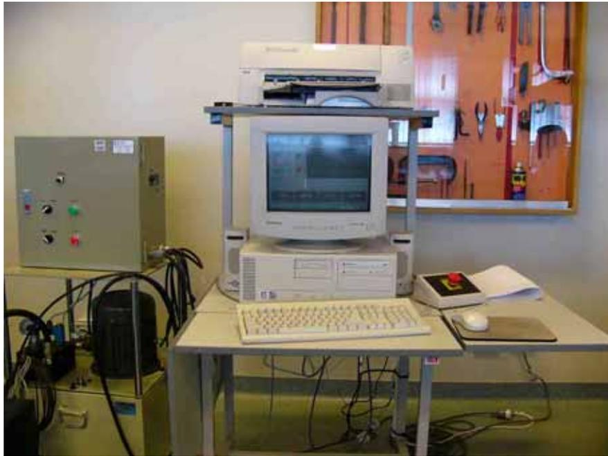
Figure 4.19: The servo system of computerised ‘Avery’ testing machine.
