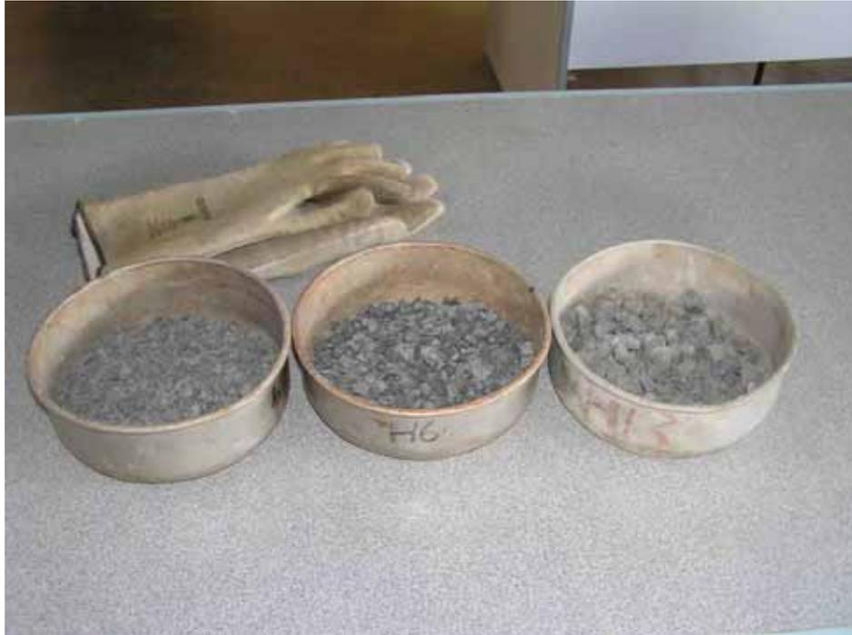
Figure 3.3: Placement of aggregates in the container before oven drying.
