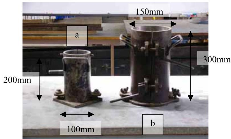
Figure 4.7: 100mm diameter x 200mm (a) and 150mm diameter x 300mm (b) cylindrical moulds.
