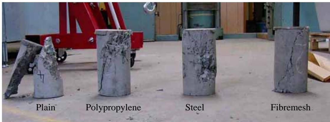
Figure 5.21: Specimens after the modulus of elasticity test.
