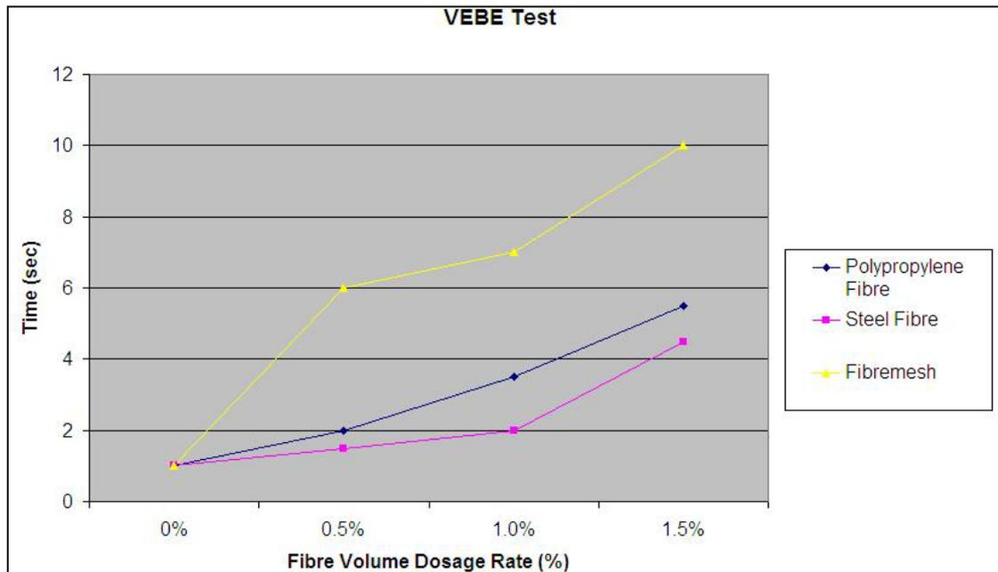
Figure 5.4: Average VEBE time vs. fibre volume dosage rate of each batch.
