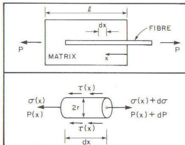
Figure 2.4: Pullout geometry to simulate the interaction between fibre and cement matrix. (Source: Bentur and Mindness, 1990)
