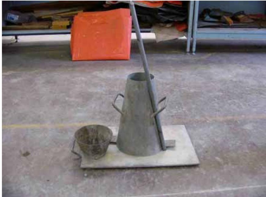
Figure 4.1: Apparatus for slump test.
