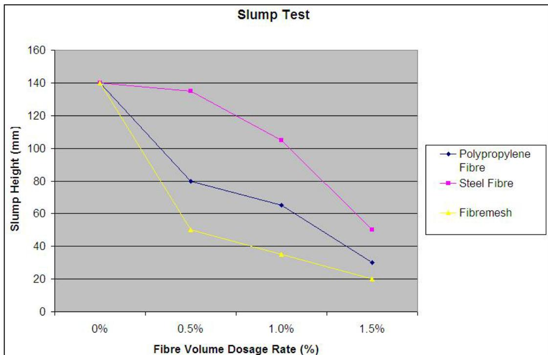
Figure 5.1: Average slump height vs. fibre volume dosage rate of each batch.
