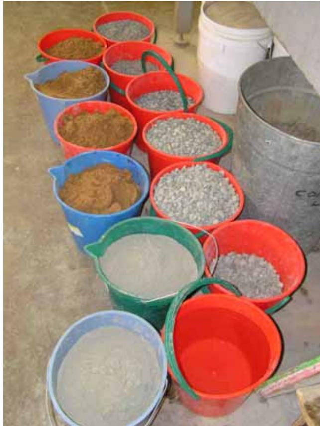
Figure 3.13: The preparation of the mixing material in the buckets.
