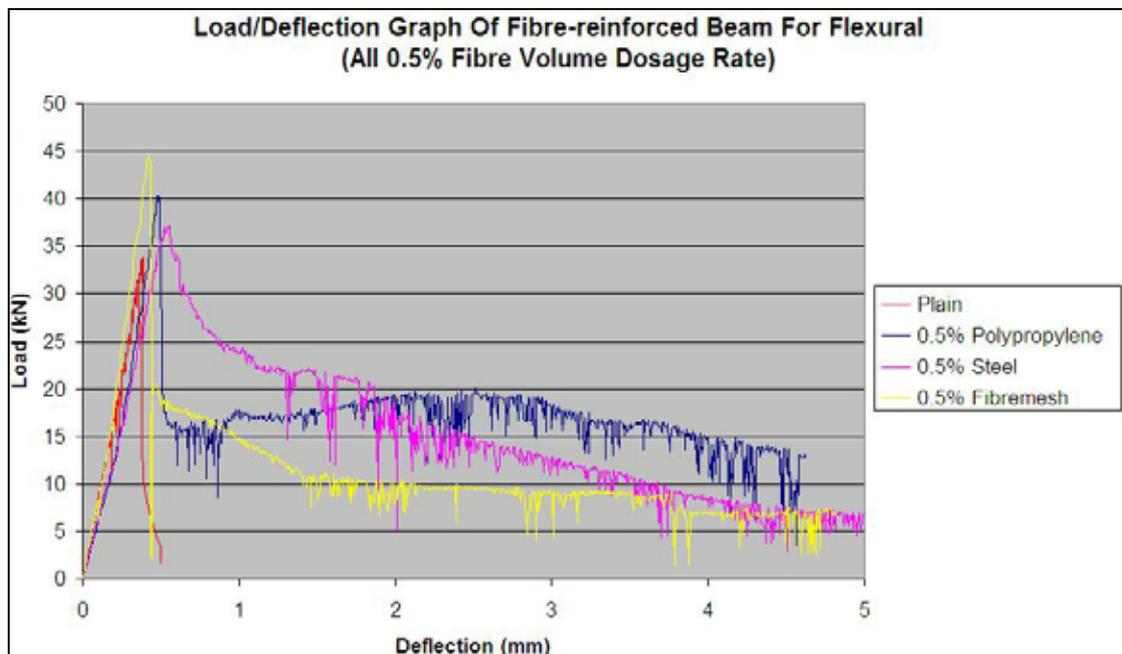
Figure 5.16: Load/deformation curves for concrete containing 0.5% fibre volume dosage rate of different type of fibres.
