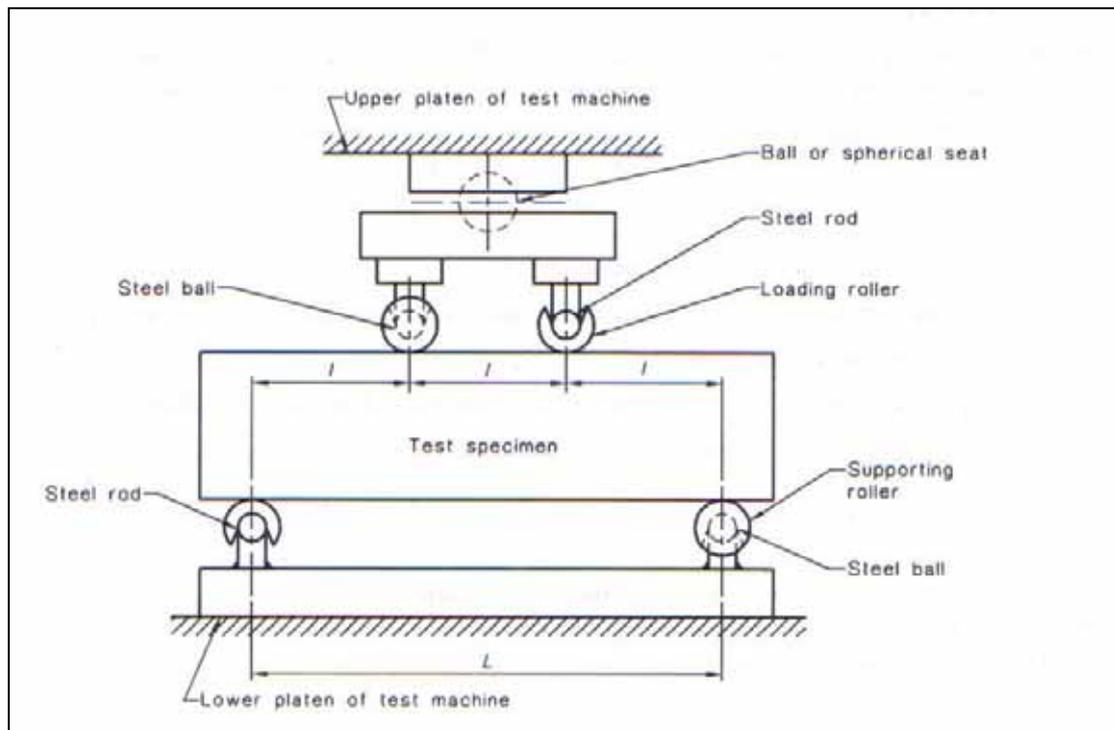
Figure 4.18: The flexural strength test. (Source: Australian Standard - AS1012, 2003)
