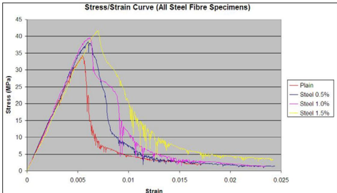
Figure 5.22: Stress/strain relationship curves for concrete containing varying amounts of steel fibres.
