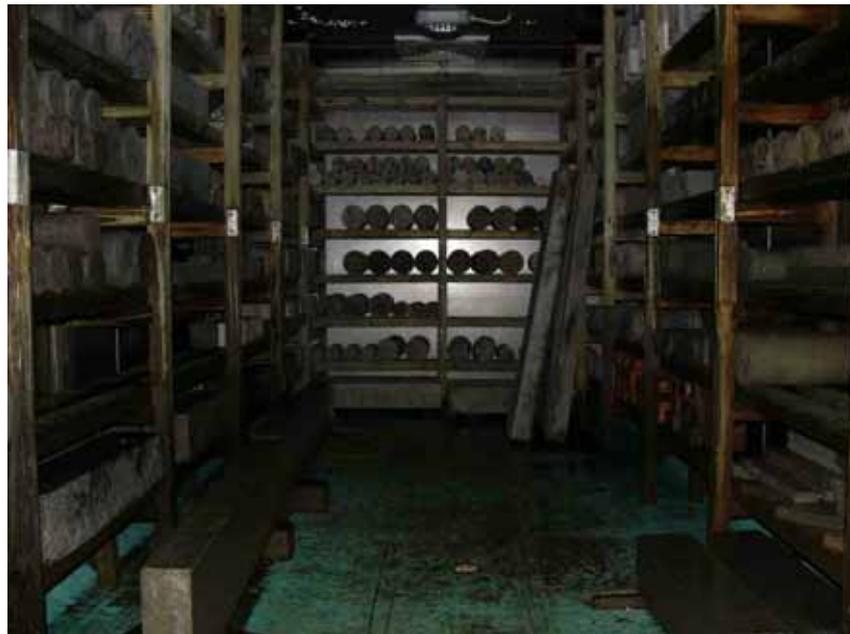
Figure 4.14: Curing of concrete specimen in curing room.
