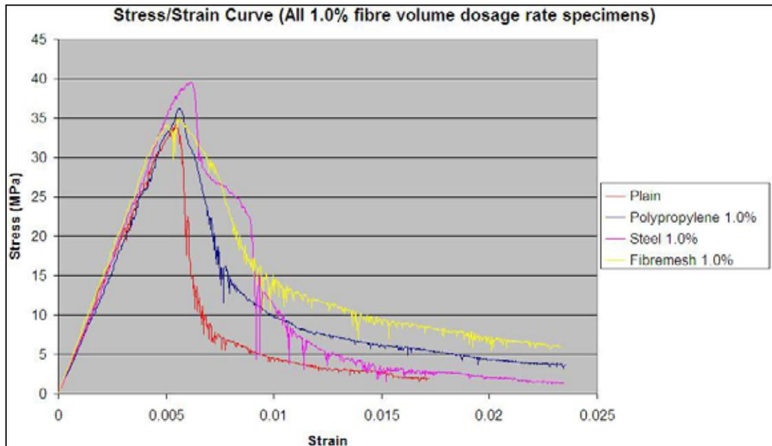
Figure 5.26: Stress/strain relationship curves for concrete containing 1.0% fibre volume dosage rate of different type of fibres.
