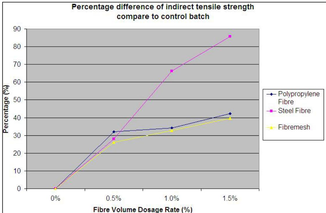
Figure 5.8: Percentage difference of indirect tensile strength vs. fibre volume dosage rate of each batch.
