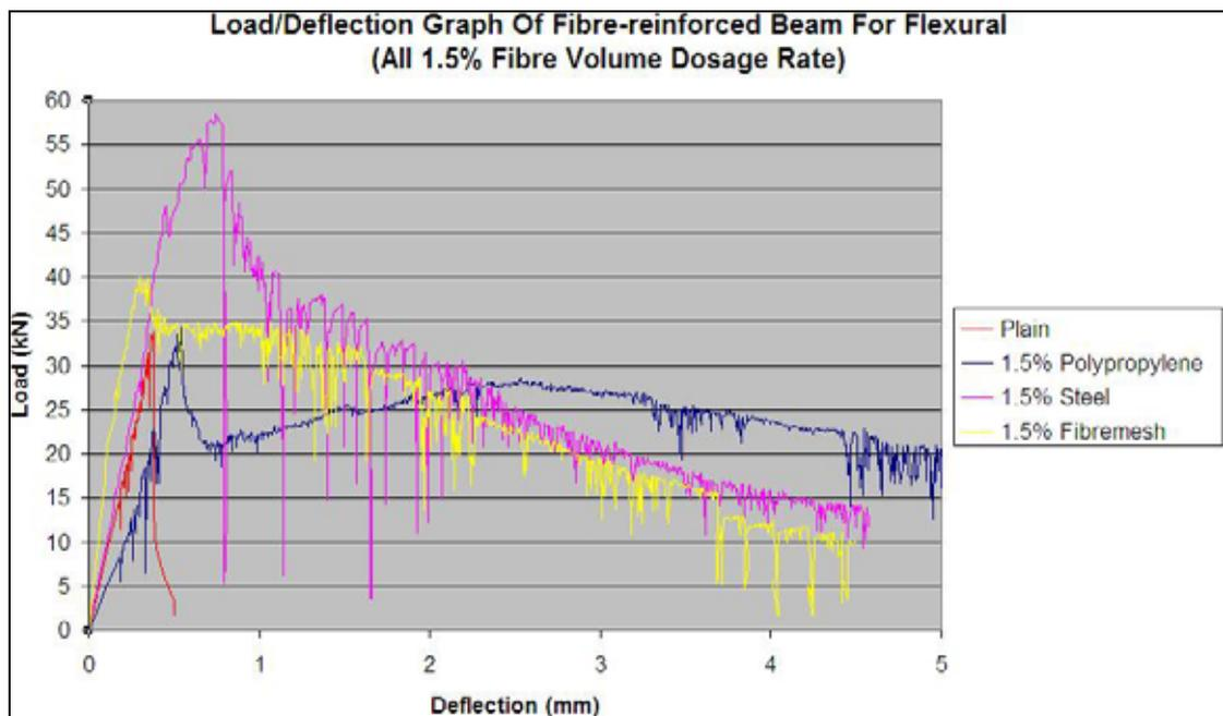
Figure 5.18: Load/deformation curves for concrete containing 1.5% fibre volume dosage rate of different type of fibres.
