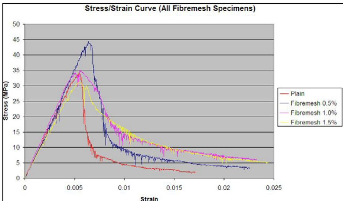
Figure 5.24: Stress/strain relationship curves for concrete containing varying amounts of Fibremesh.
