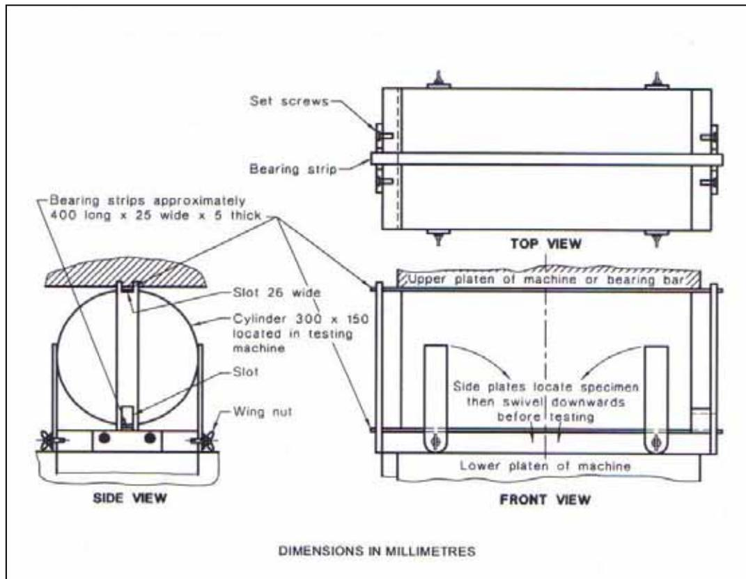
Figure 4.16: Apparatus of indirect tensile strength test with dimension.
