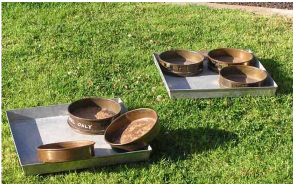
Figure 3.6: Drying of wet natural sand was under the sun.
