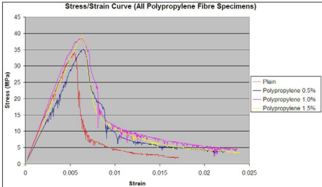
Figure 5.23: Stress/strain relationship curves for concrete containing varying amounts of polypropylene fibres.
