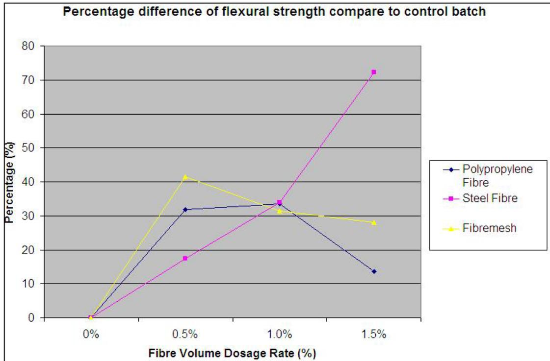
Figure 5.11: Percentage differences of flexural strength vs. fibre volume dosage rate for each batch.
