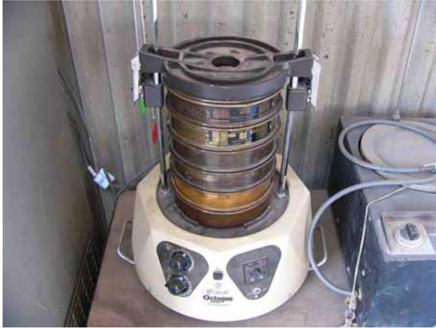
Figure 3.9: Mechanical sieve machine for fine aggregates.
