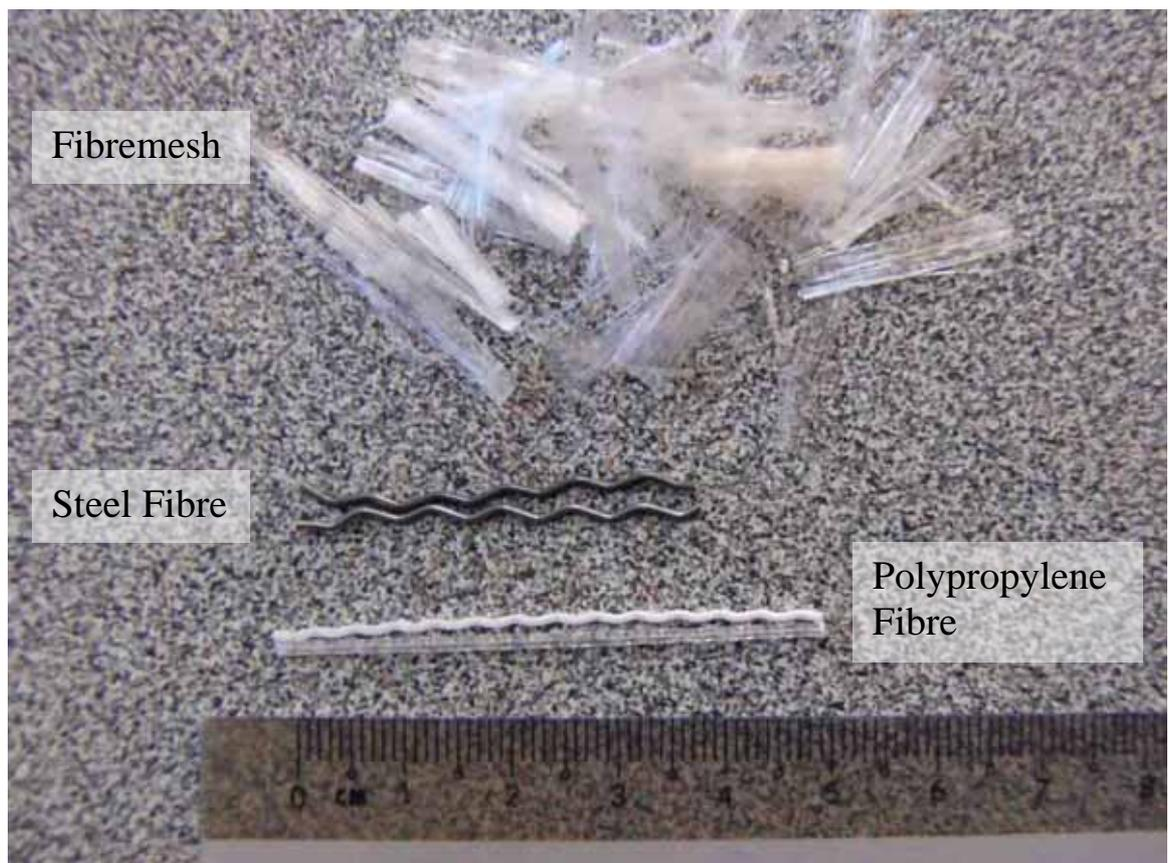
Figure 3.11: Types of fibre used in the concrete mix.
