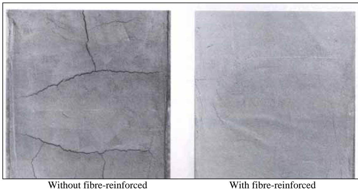
Figure 1.3: Comparison of cracks with and without Fibre reinforced.
