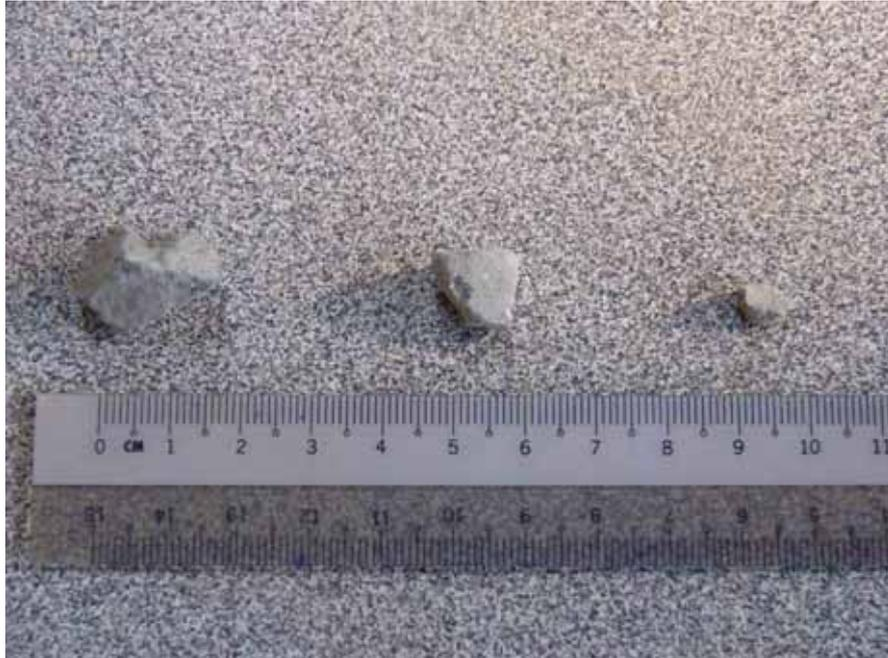
Figure 3.1: Natural aggregate size from 20mm, 10mm and 7mm.
