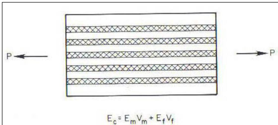
Figure 2.11: The parallel model of 'rule of mixture'.
