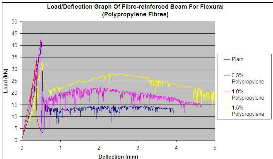
Figure 5.14: Load/deformation curves for concrete containing varying amounts of polypropylene fibres.
