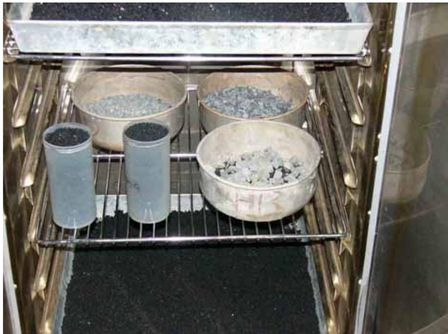
Figure 3.4: The thermostatically controlled oven.
