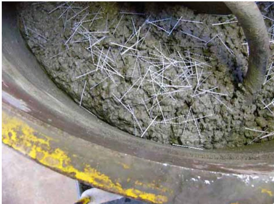
Figure 3.14: Additional of fibres after the main materials were mixed.
