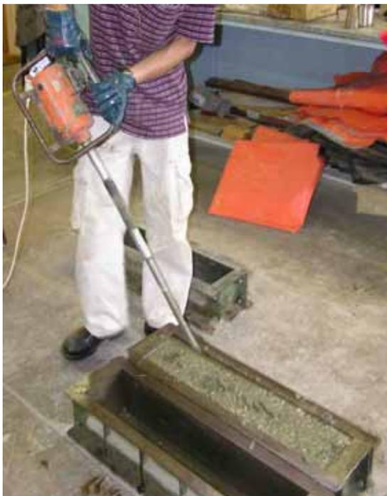
Figure 4.10: Use of immersion vibrator.
