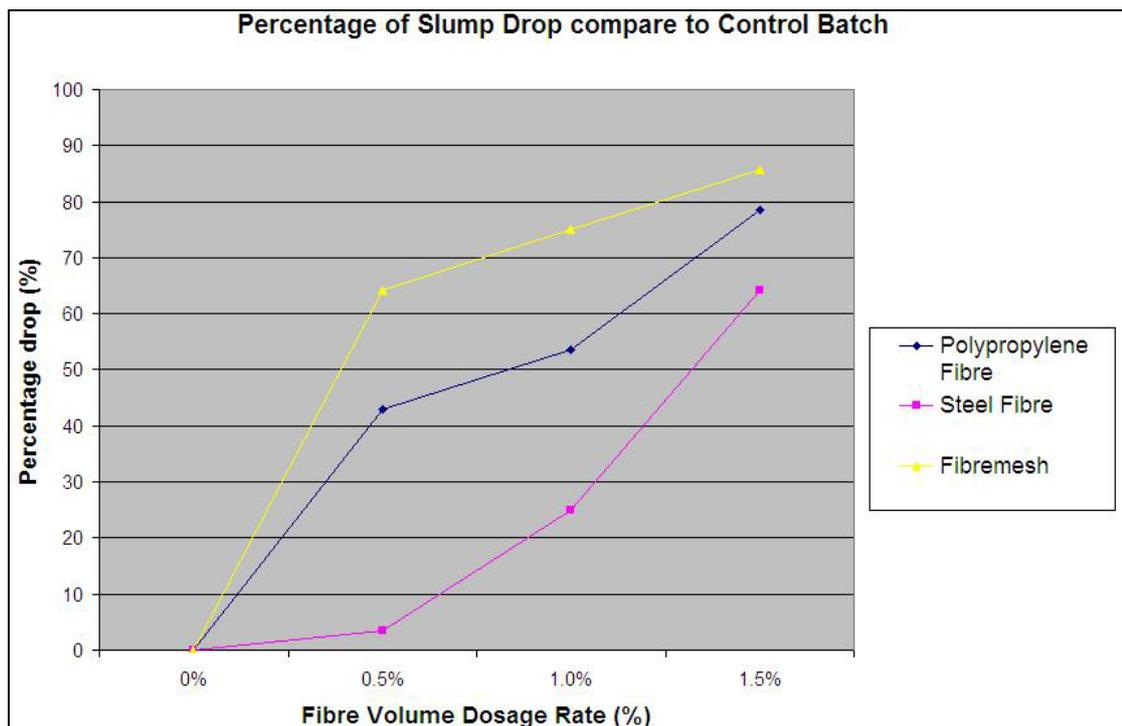
Figure 5.2: Percentage drop of slump vs. fibre volume dosage rate of each batch.
