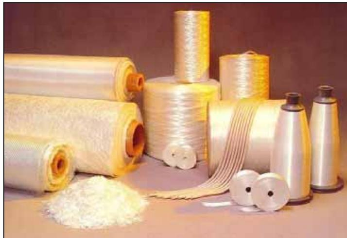
Figure 1.8: Drums of glass fibre strands. (Source: J&J Trading Corp, 2002)
