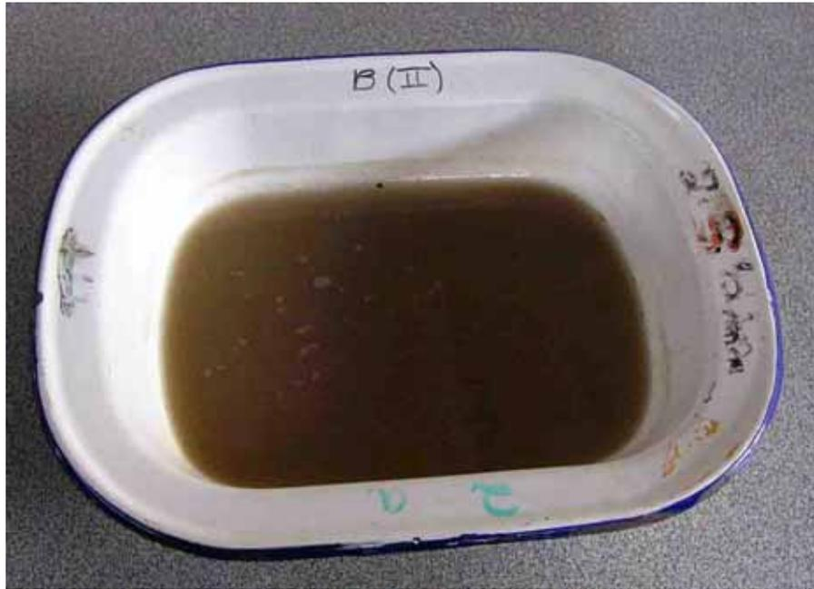
Figure 3.7: Placement of natural sand in the container before oven drying.
