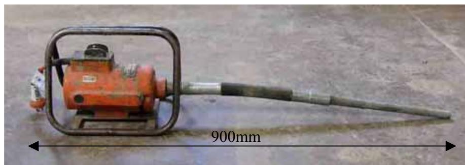
Figure 4.9: An immersion vibrator.
