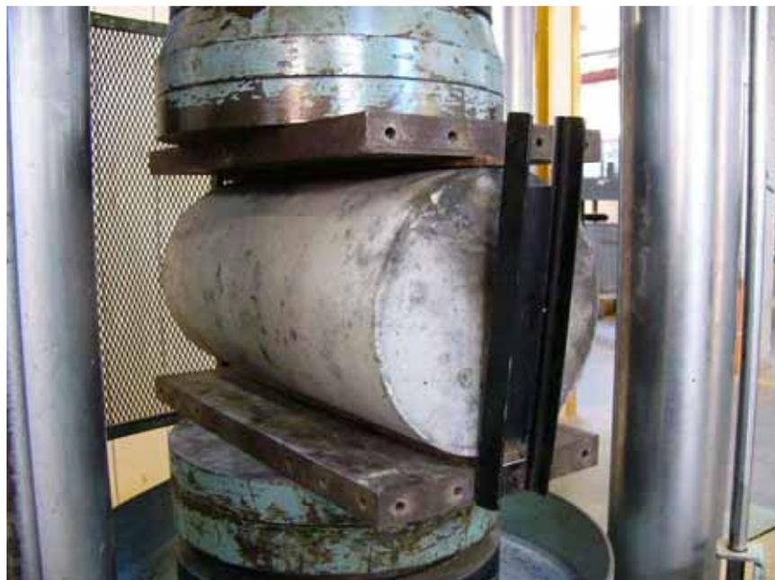
Figure 4.17: A typical set up of indirect tensile test.
