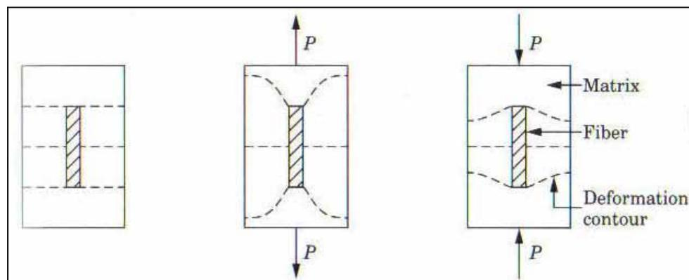
Figure 2.5: Interaction of fibre-uncracked matrix.
