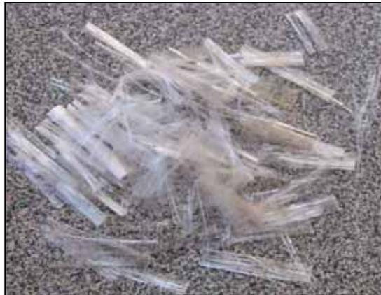
Figure 1.10: Mesh geometry of synthetic fibres. (Film type)
