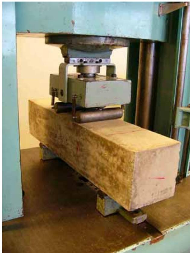
Figure 4.20: A typical flexural strength tests under 4-point loading.
