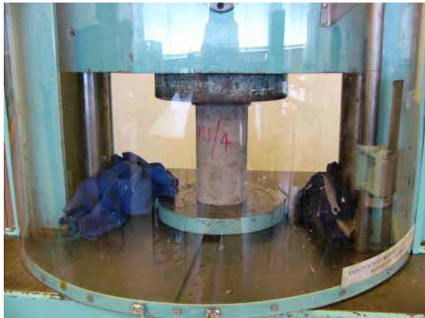
Figure 4.22: A typical test for modulus of elasticity.
