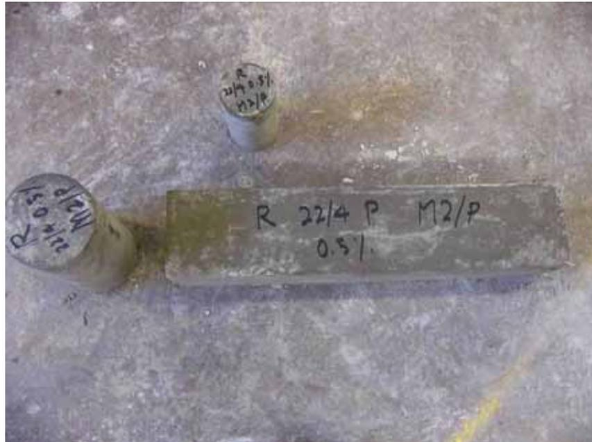
Figure 4.13: Concrete specimen after stripping.
