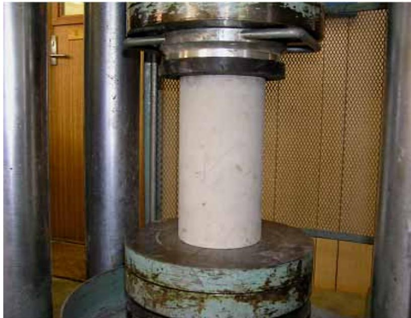
Figure 4.15: A typical compression test of 100mm diameter x 150mm height concrete specimen with rubber capping.
