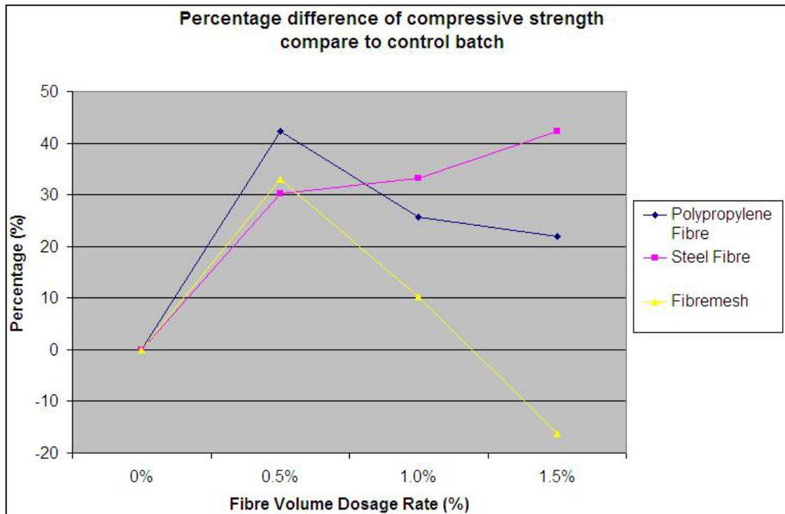
Figure 5.6: Percentage difference of compressive strength vs. fibre volume dosage rate of each batch.
