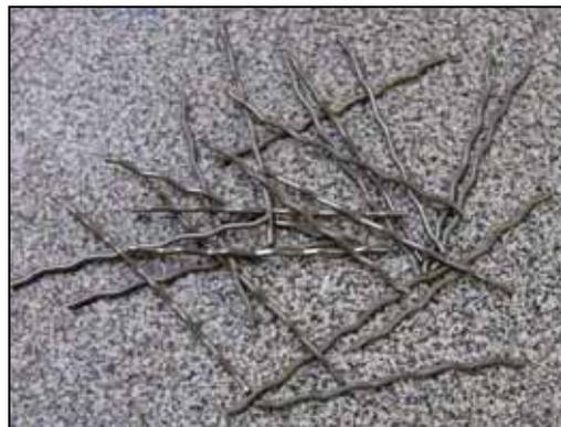
Figure 1.4: Wave-cut steel fibres.
