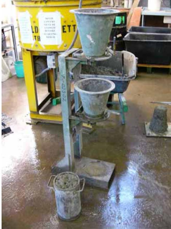
Figure 4.4: The compacting factor test. The concrete in the cylinder mould is about to measure for its weight.
