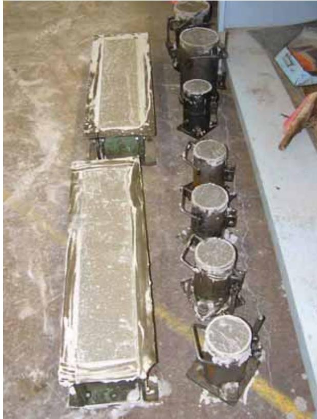
Figure 4.12: The concrete specimens in the mould after 24 hours.
