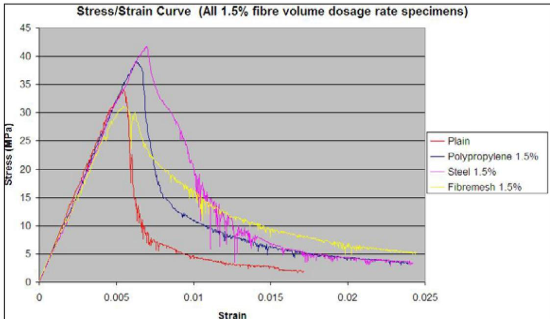
Figure 5.27: Stress/strain relationship curves for concrete containing 1.5% fibre volume dosage rate of different type of fibres.
