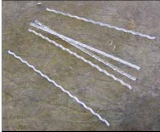
Figure 1.9: Twisted wave geometry of synthetic fibres. (Monofilament type)
