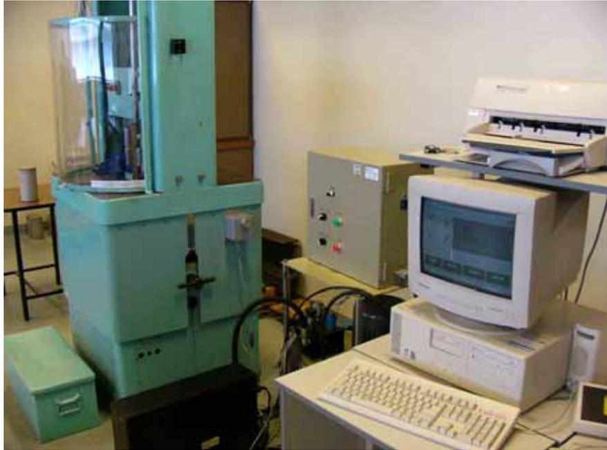
Figure 4.21: Computerised 'Avery' testing machine.
