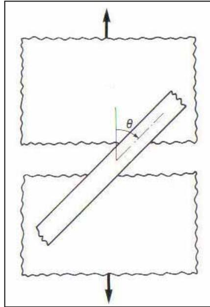
Figure 2.8: The intersection of an oriented fibre across a crack with an angle ( $\theta$ ).
