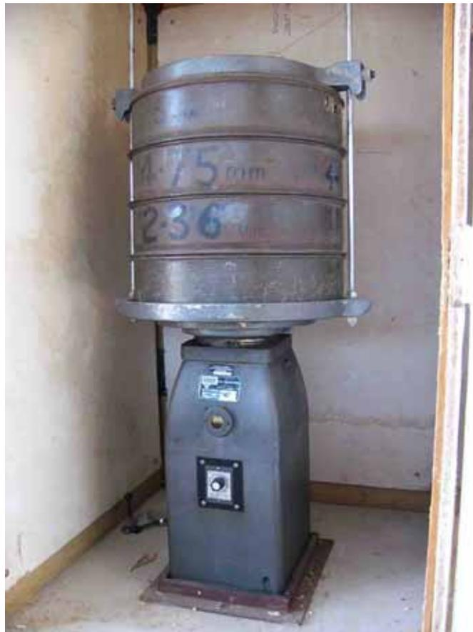
Figure 3.10: Mechanical sieve machine for coarse aggregate.
