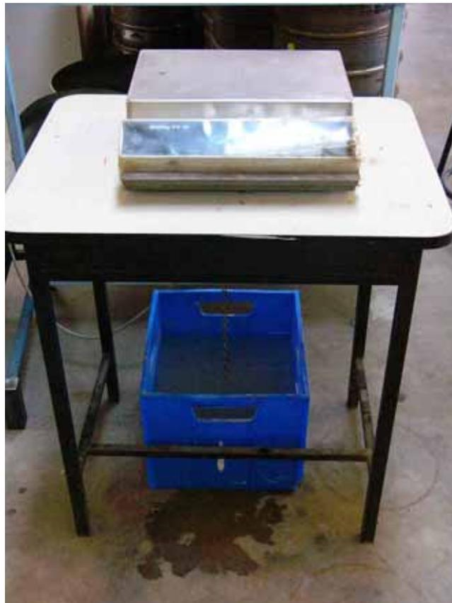
Figure 3.2: Immersion of aggregates and wire basket into the water for weight record.
