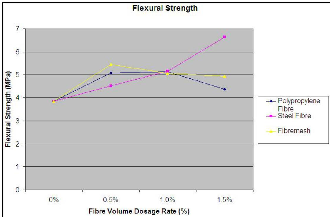
Figure 5.10: Average flexural strength vs. fibre volume dosage rate of each batch.
