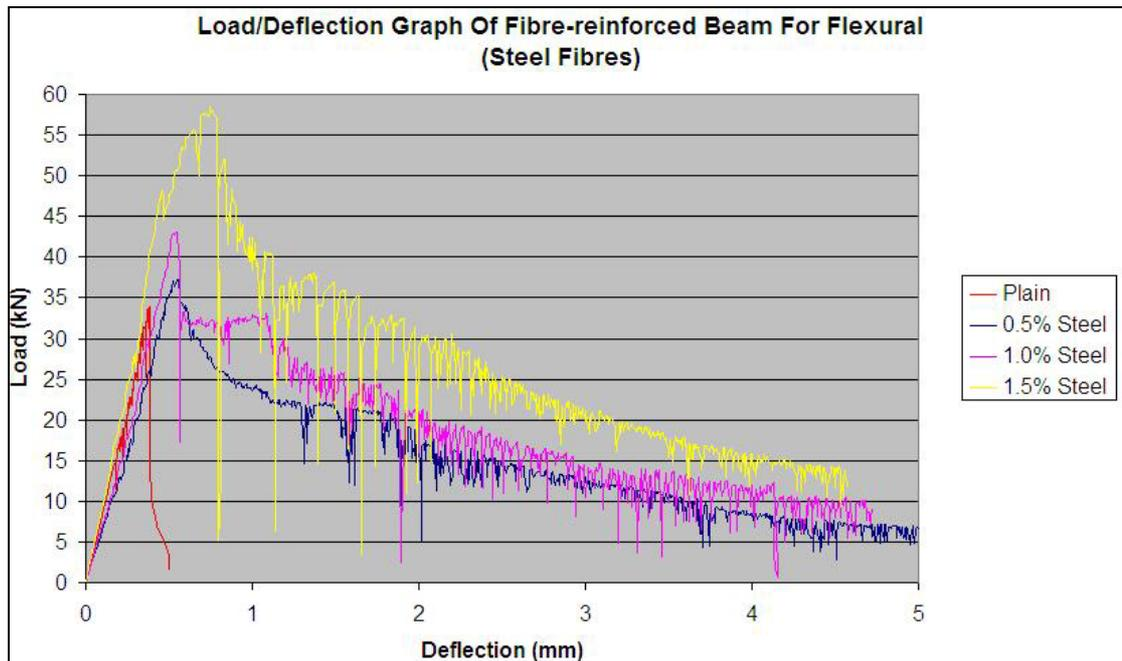
Figure 5.13: Load/deformation curves for concrete containing varying amounts of steel fibres.
