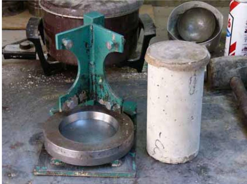
Figure 4.23: Mould used to form sulphur cap for specimens.
