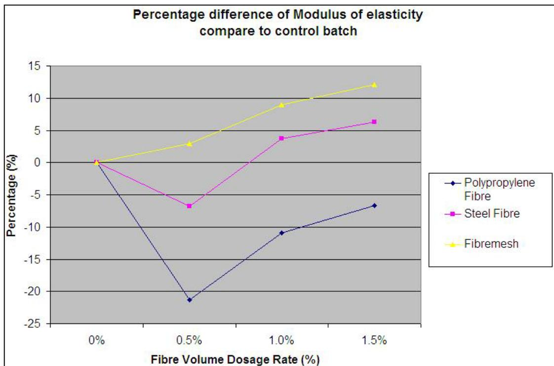
Figure 5.20: Percentage differences of modulus of elasticity vs. fibre volume dosage rate for each batch.
