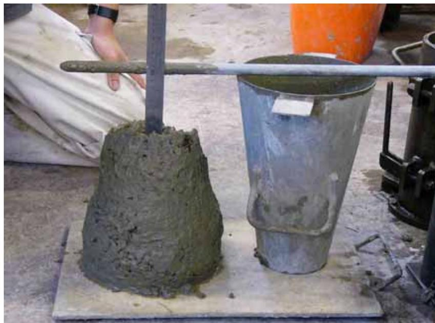
Figure 4.2: A typical slump test.
