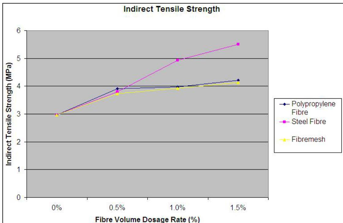
Figure 5.7: Average indirect tensile strength vs. fibre volume dosage rate of each batch.
