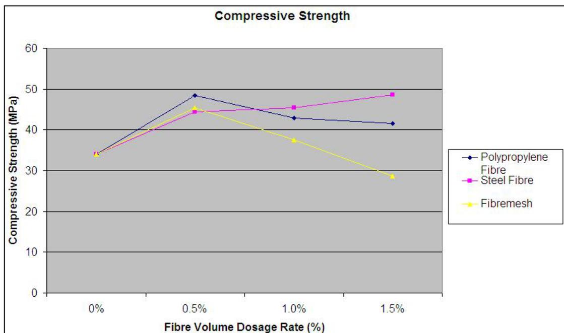
Figure 5.5: Average compressive strength vs. fibre volume dosage rate of each batch.
