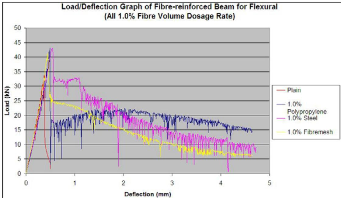
Figure 5.17: Load/deformation curves for concrete containing 1.0% fibre volume dosage rate of different type of fibres.
