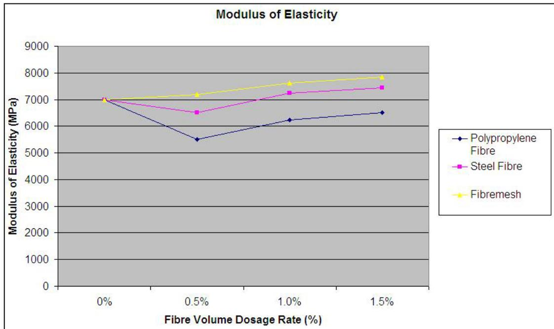
Figure 5.19: Average modulus of elasticity vs. fibre volume dosage rate of each batch.
