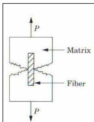
Figure 2.6: Interaction of fibre-cracked matrix.
