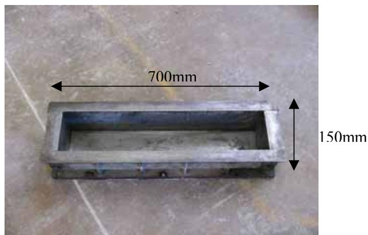
Figure 4.8: Beam mould with dimensions of 150mm x 150mm x 700mm.
