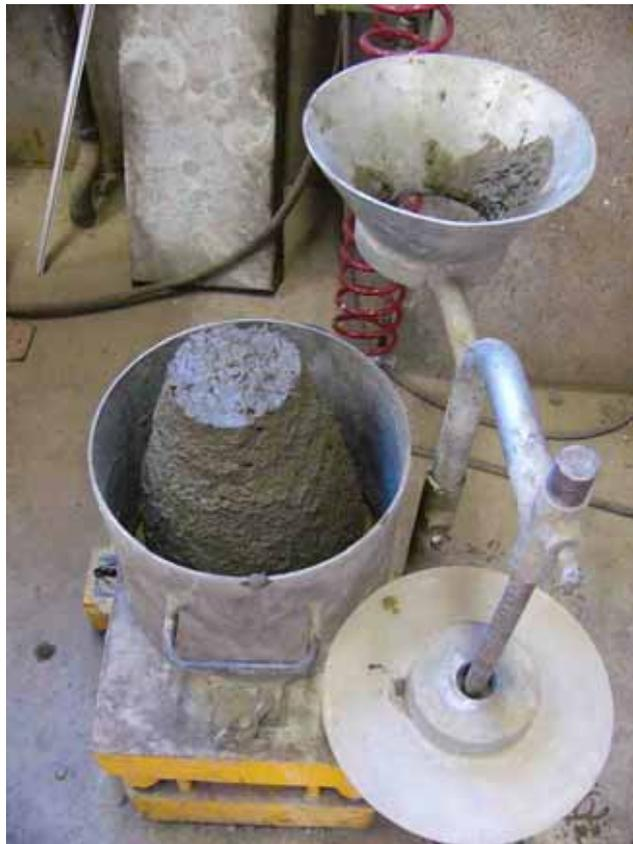
Figure 4.6: The VEBE consistometer test. The concrete in the mould is positioned before the disc is placed.
