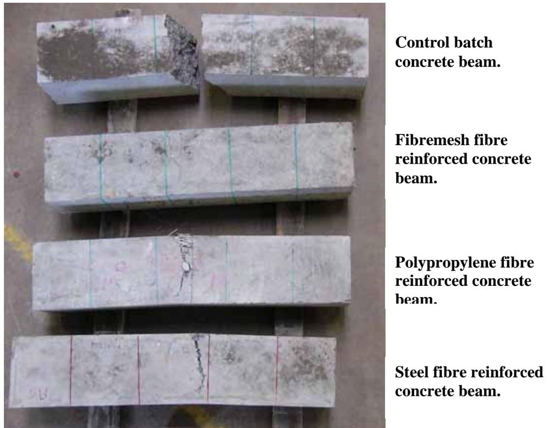
Figure 5.12: Concrete beam specimen after the tests.
