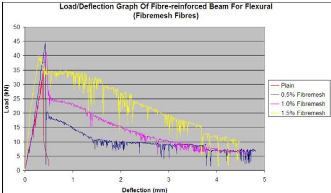
Figure 5.15: Load/deformation curves for concrete containing varying amounts of Fibremesh.
