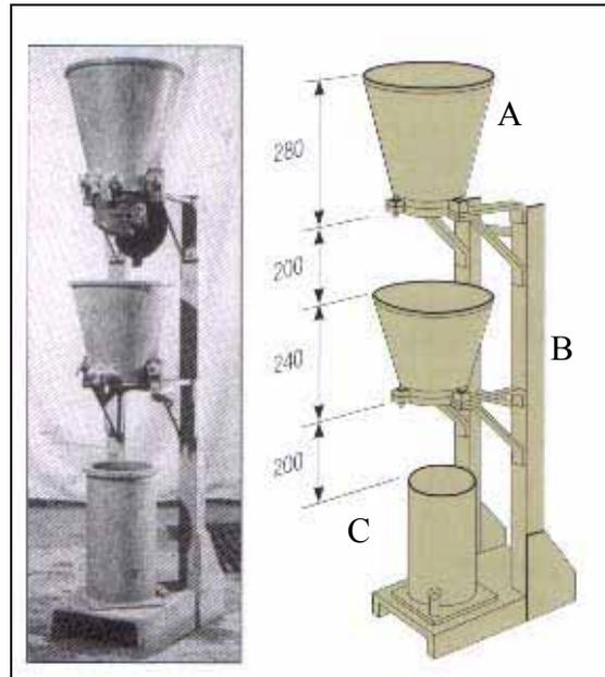
Figure 4.3: Apparatus for compacting factor tests. (Source: Australian Standard HB64, 2002)
