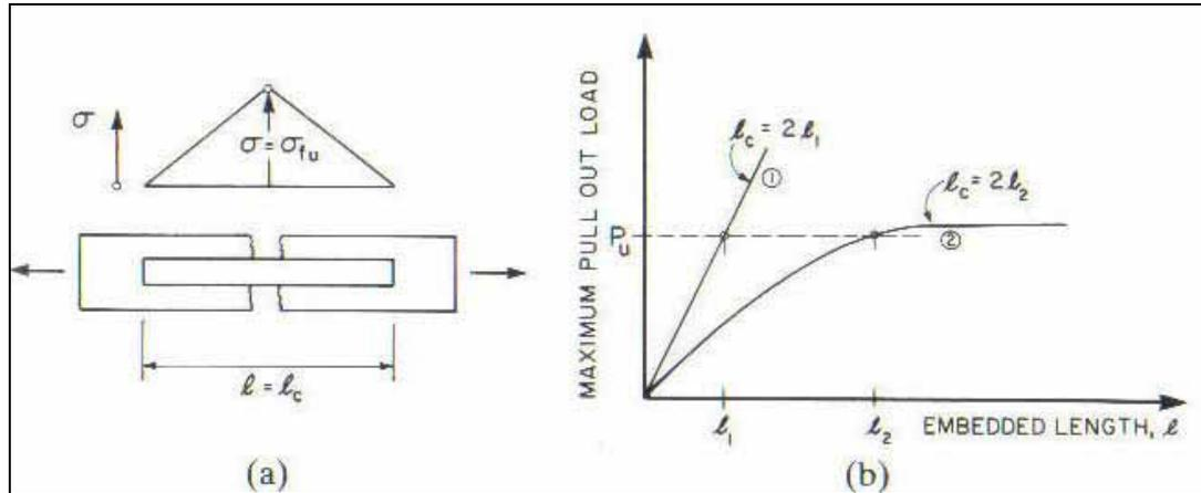
Figure 2.7: Definition of critical length: (a) Frictional stress distribution on fibres. (b) Intersection of fibre breaking load  $P_u$ , with pullout load versus embedded length. (Source: Bentur and Mindness, 1990)
