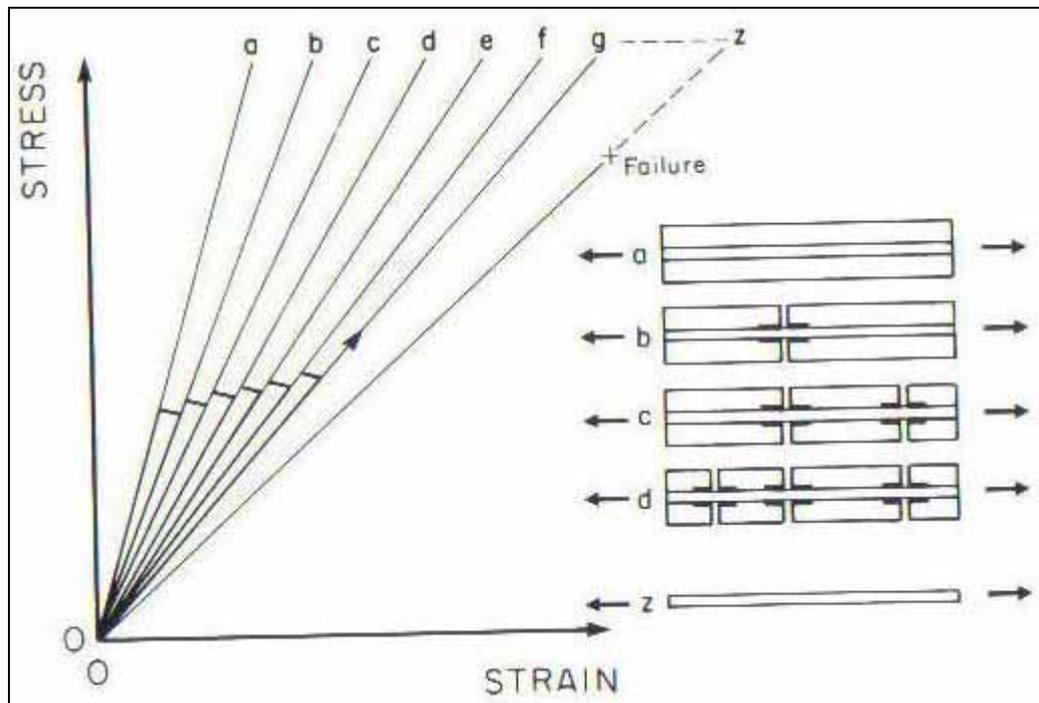
Figure 2.9: The multiple cracking process and the stages of stress/strain curve related to the multiple cracking processes. (Source: Bentur and Mindness, 1990)
