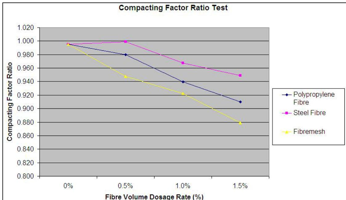
Figure 5.3: Average compacting factor ratio vs. fibre volume dosage rate of each batch.
