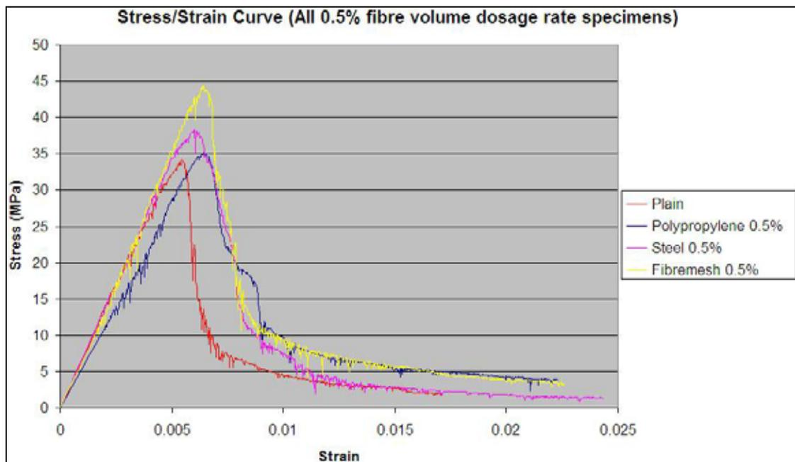
Figure 5.25: Stress/strain relationship curves for concrete containing 0.5% fibre volume dosage rate of different type of fibres.
