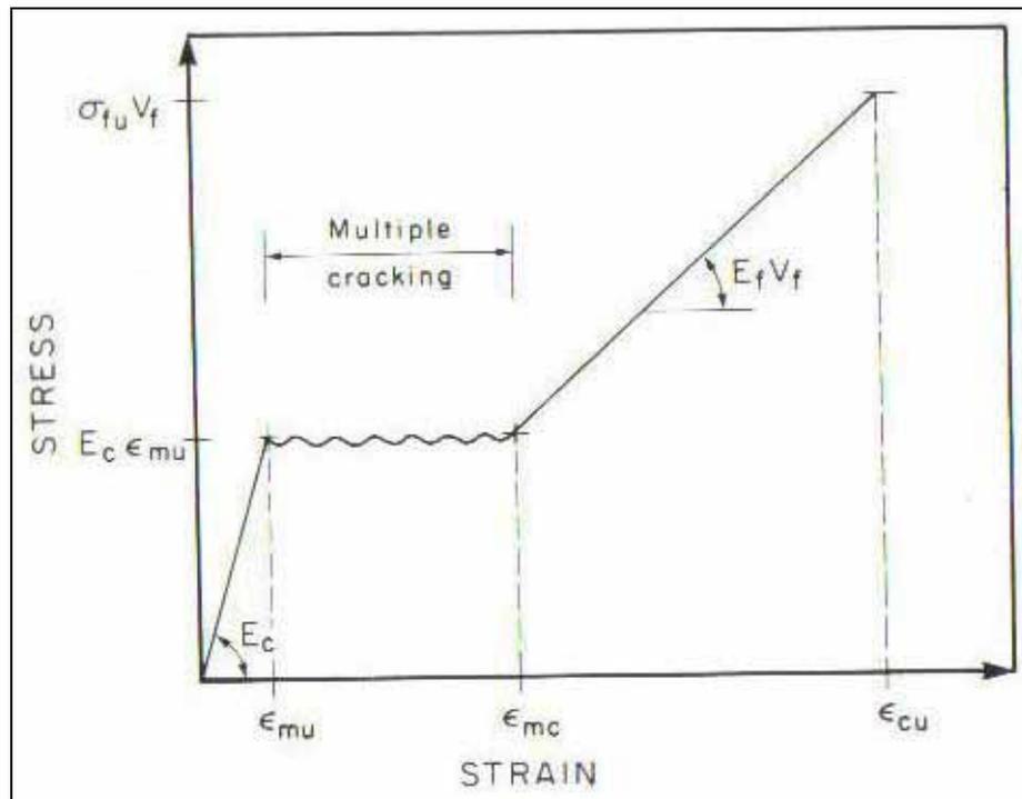
Figure 2.10: Final schematic description of stress/strain curve.
