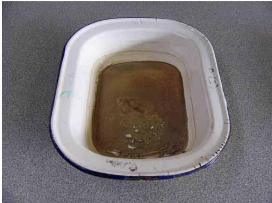
Figure 3.8: Natural sand in the container after oven drying.
