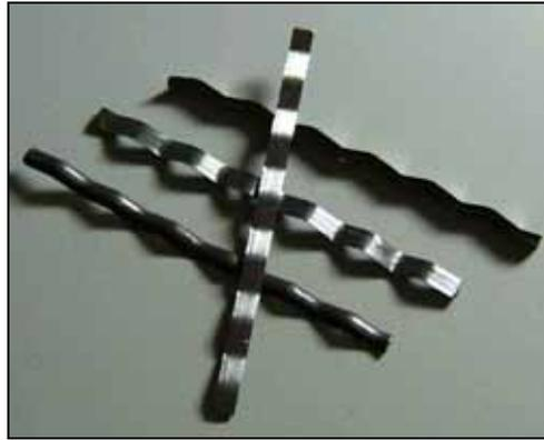
Figure 1.6: Deformed sheet steel fibres.
