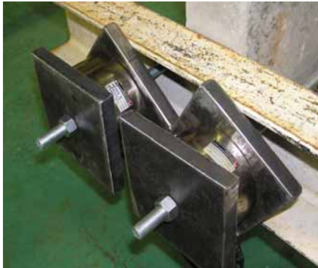
Figure 4.14(a) Load Cells on dead anchorage end
