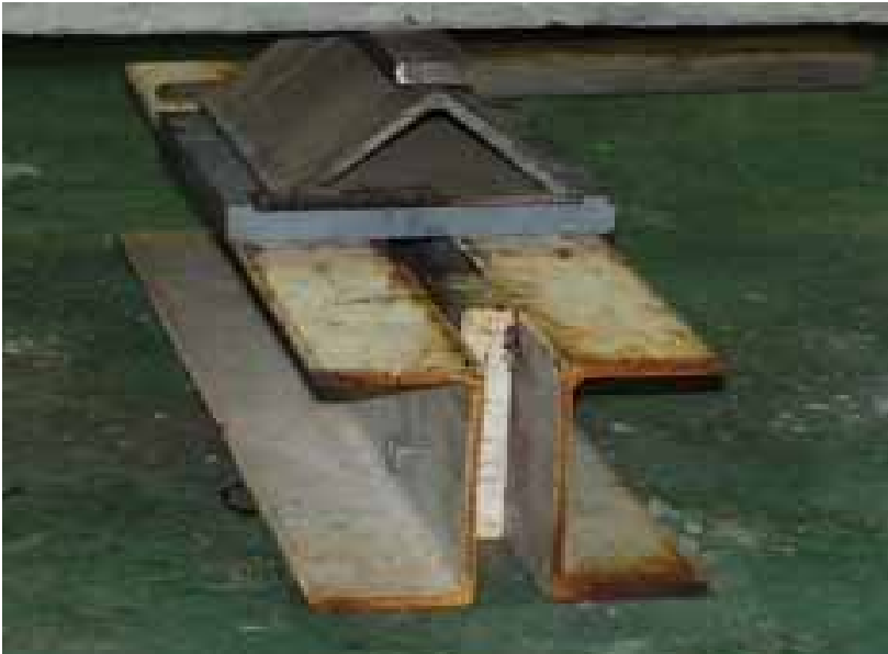
Figure 4.11: Main support arrangement for girders.
