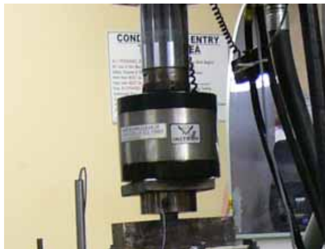
Figure 4.14(b): Load Cells under the loading ram of Instron Machine
