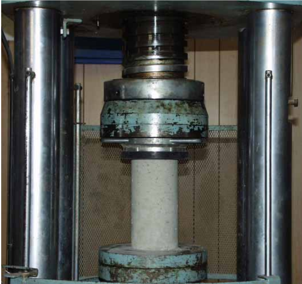
Figure 5.1: Cylinder Compression Test (Avery Testing Machine)
