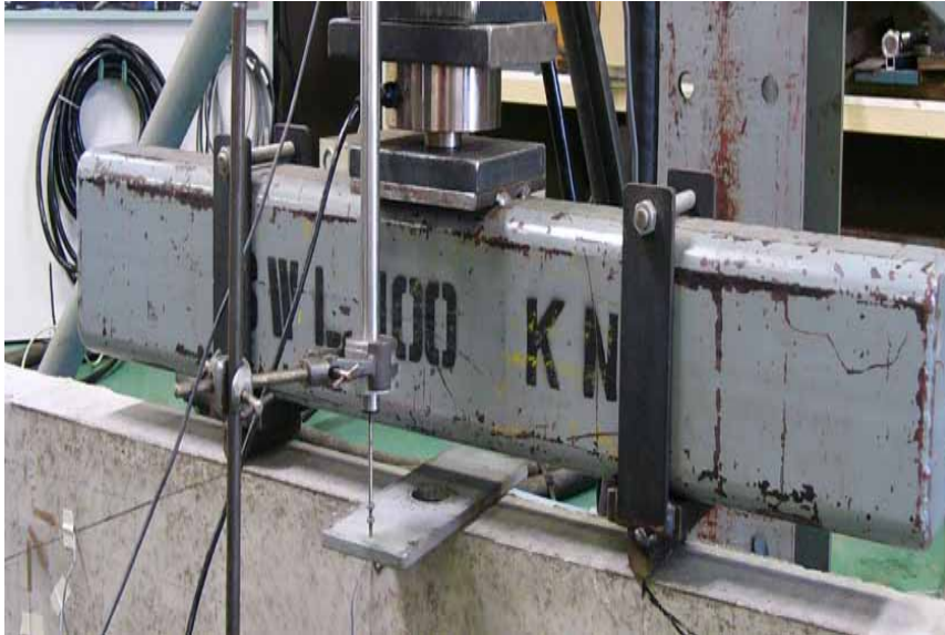
Figure 4.12: Placement of Spreader beam on concrete girders.
