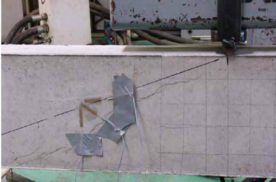
Figure 5.8: Preloading Crack Pattern of Beam B2
