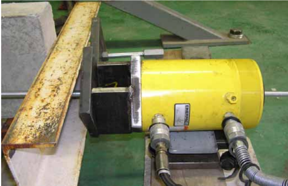
Figure 4.18: Post-tensioning jack stressing threaded rods.
