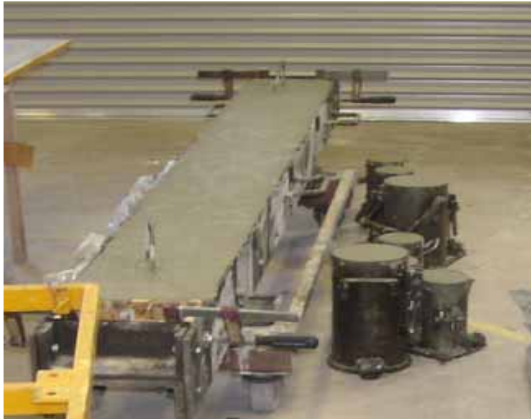
Figure 4.7: Recently cast specimen
