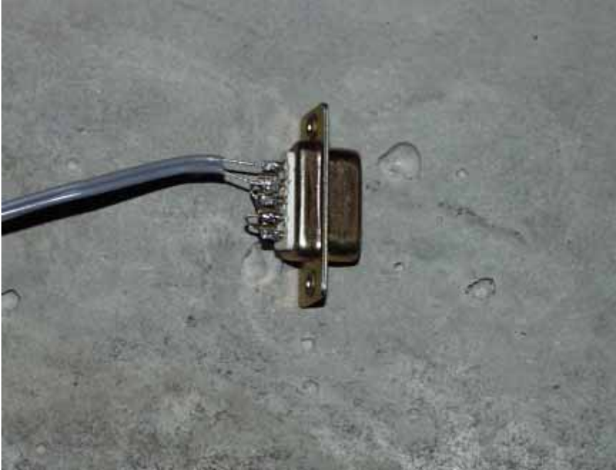
Figure 4.10: Strain gauge wires soldered with connection
