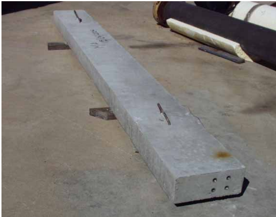
Figure 4.8: Beam after stripping
