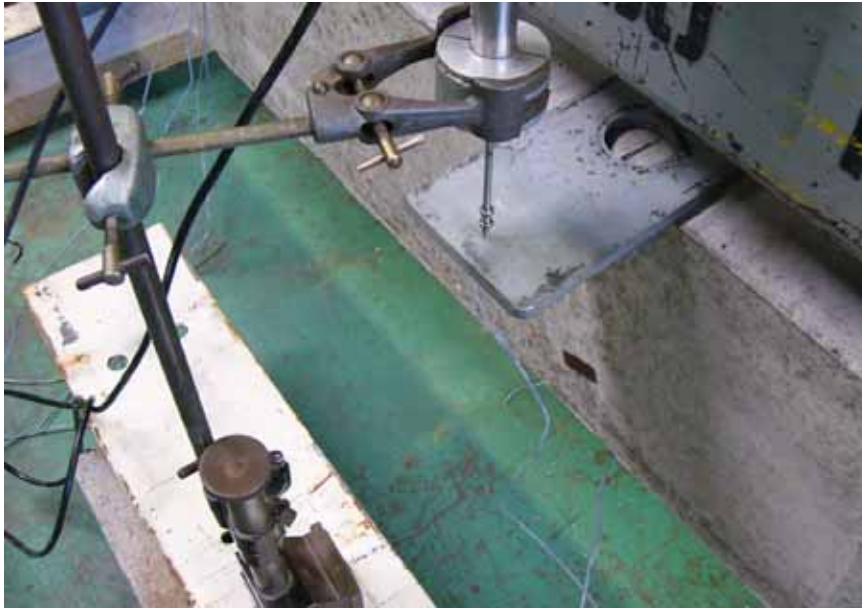
Figure 4.15: Installation of LVDT during testing of beam
