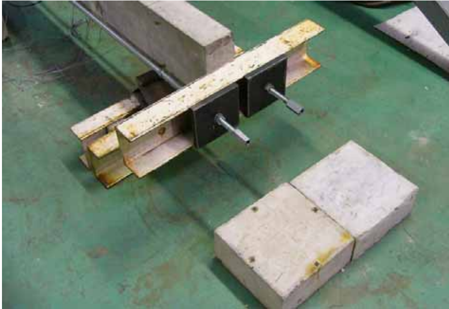
Figure 4.16: Anchoring system for post-tensioned beam.
