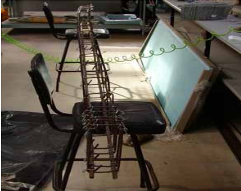
Figure 4.3: Steel Reinforcement Cage
