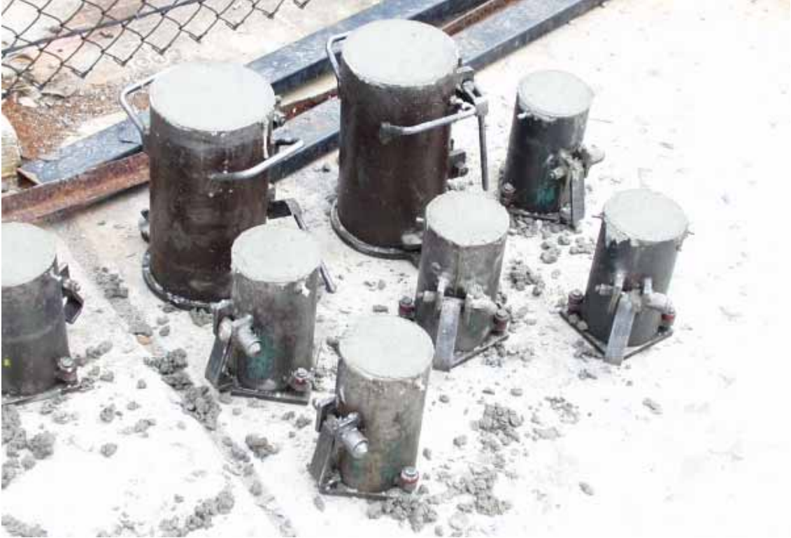
Figure 4.6: Concrete cylinders cast in moulds
