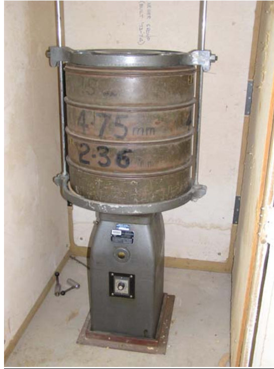
Figure 3.2: Mechanical Sieve Machine for Coarse Aggregates (Aggregates of sizes 7 mm, 10 mm, 20 mm).
